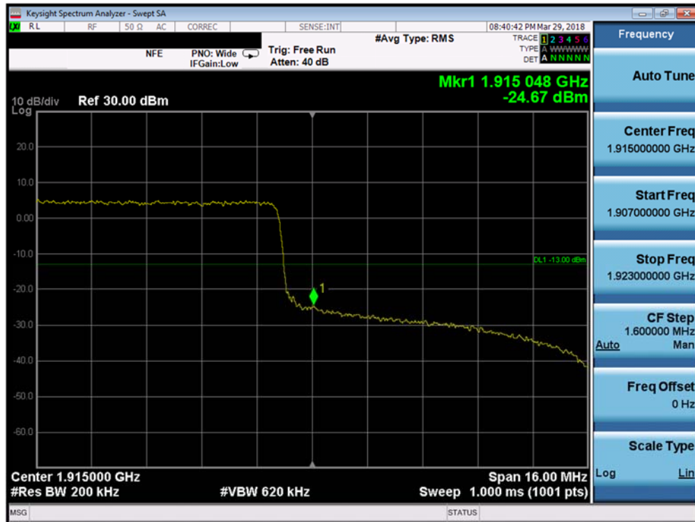
Plot 7-207. Upper Band Edge Plot (Band 25 - 20.0MHz QPSK - Full RB Configuration)
