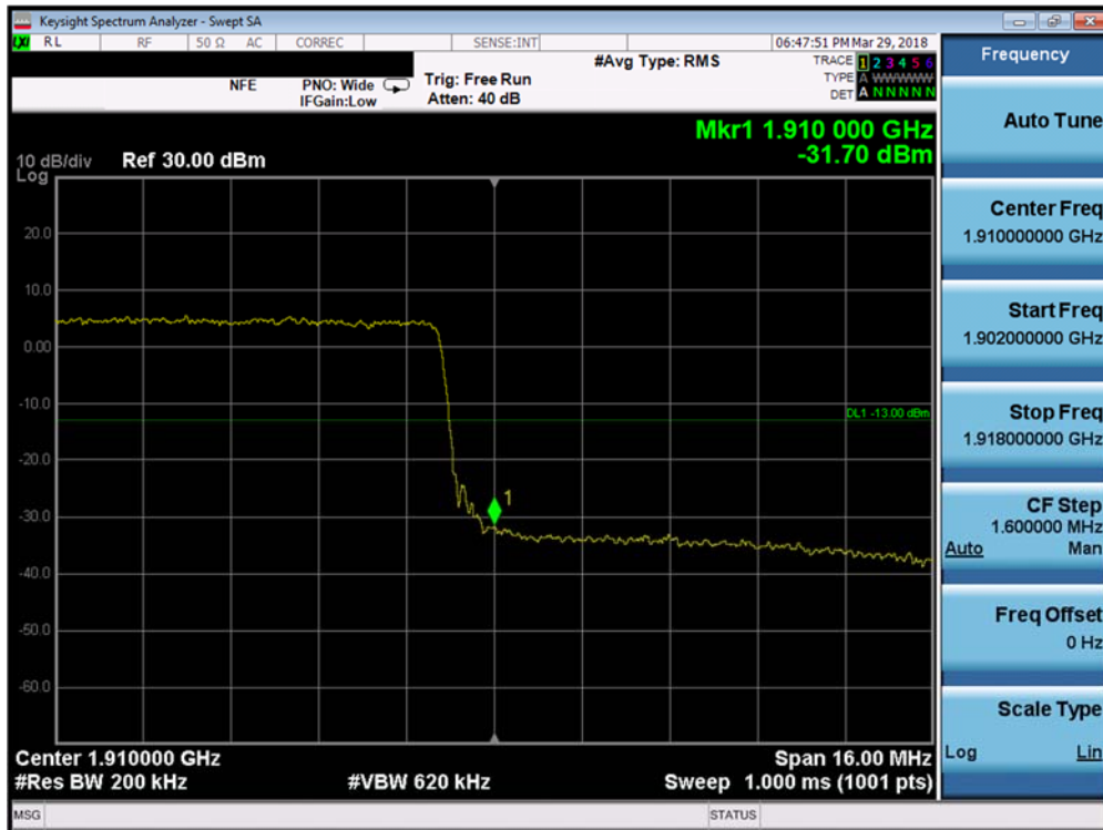
Plot 7-205. Upper Band Edge Plot (Band 2 - 20.0MHz QPSK - Full RB Configuration)
