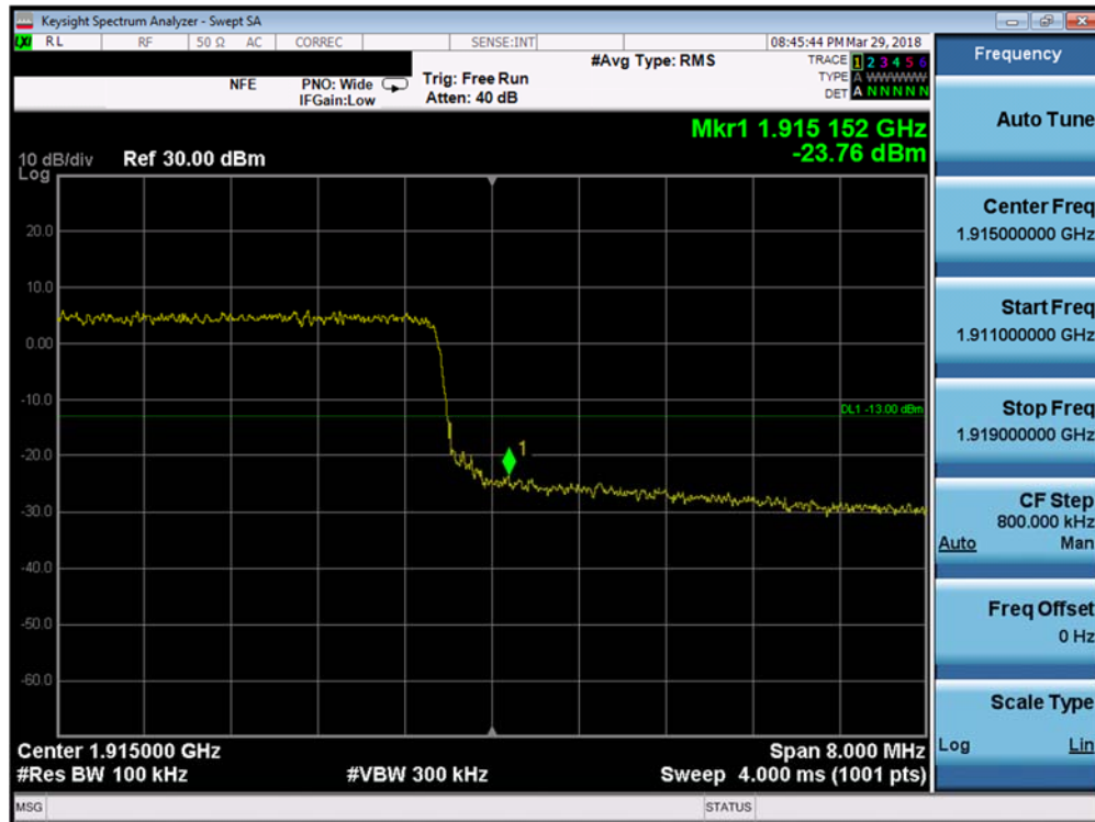
Plot 7-195. Upper Band Edge Plot (Band 25 - 10.0MHz QPSK - Full RB Configuration)
