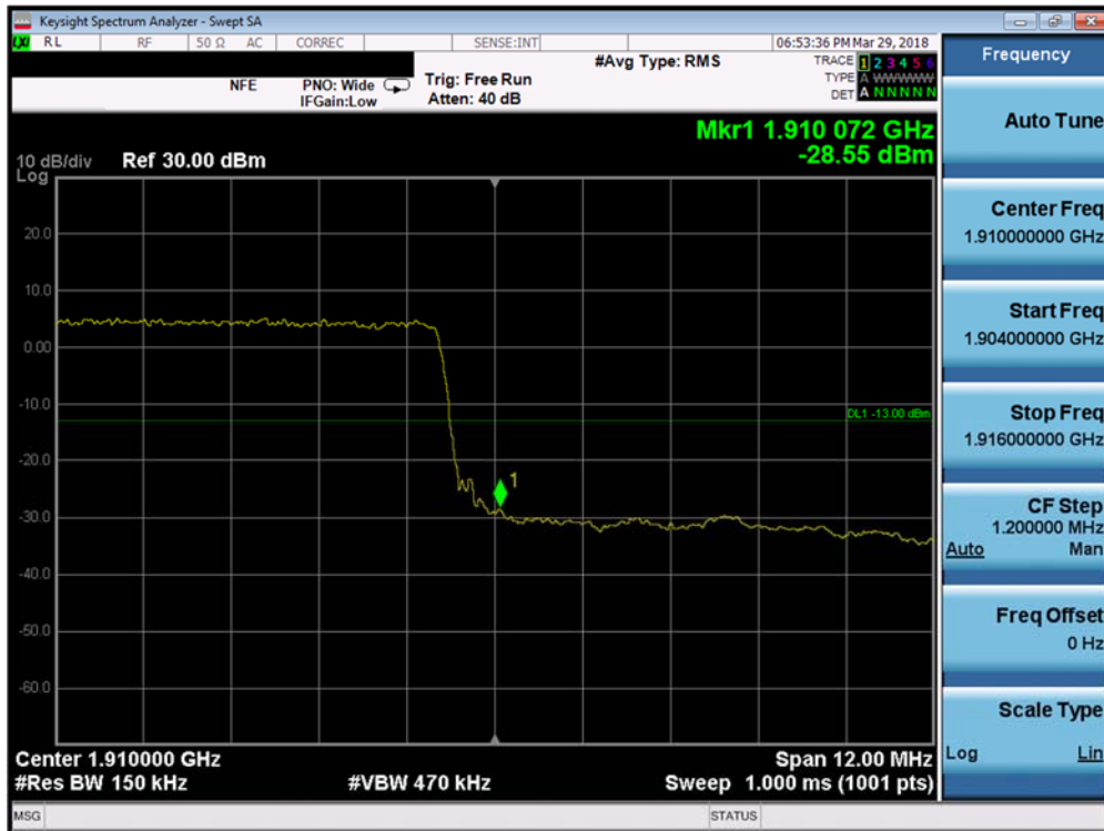
Plot 7-199. Upper Band Edge Plot (Band 2 - 15.0MHz QPSK - Full RB Configuration)
