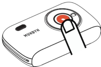
2. Take out a consumable, put it into the compartment according to the direction shown below, place your finger in the "Push" position and press it into place until it makes a "click" sound.
