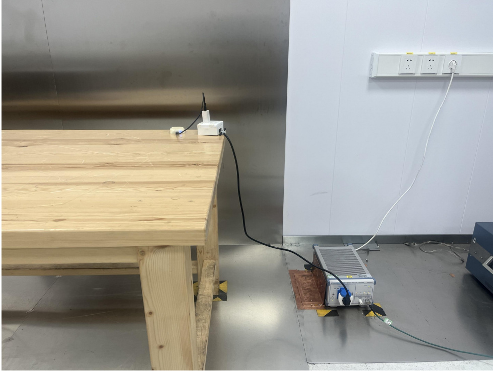
Radiated Emission Test View|(Below 1G)
