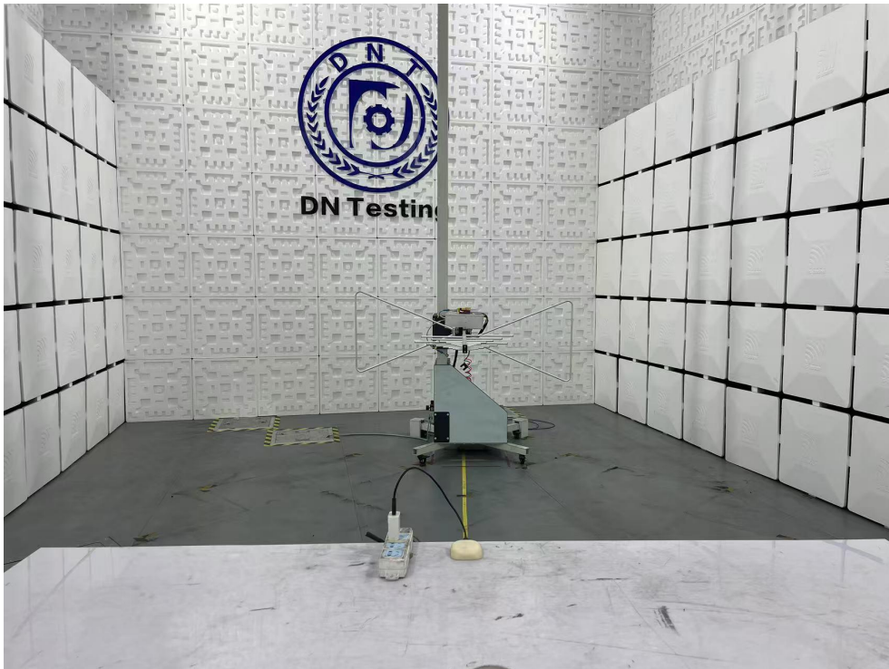
Radiated Emission Test View|(Below 1G)
