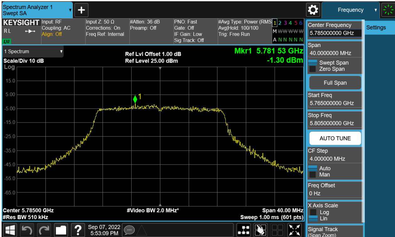
Figure 62: The plots of Power Spectral Density, 802.11n(HT20), 5825MHz, at Chain 1
