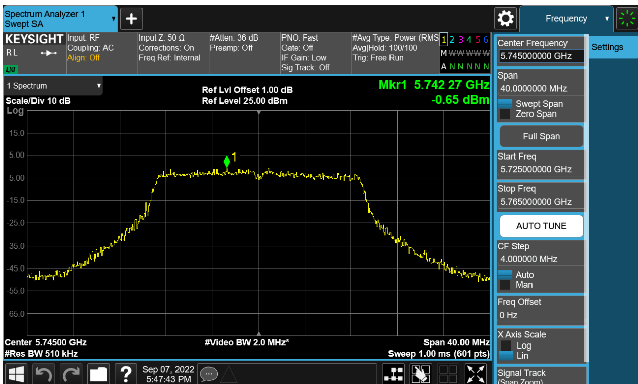
Figure 60: The plots of Power Spectral Density, 802.11n(HT20), 5745MHz, at Chain 1
