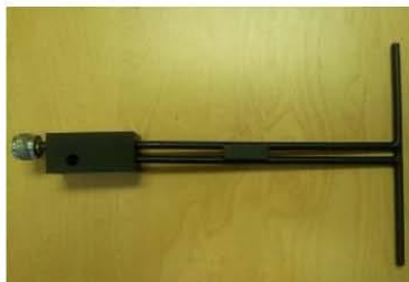
Figure 1 – MVG COMOSAR Validation Dipole
