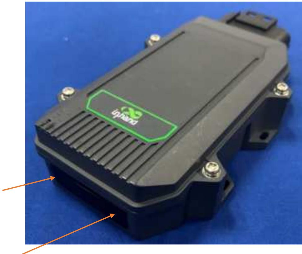
Arrow position for SIM card cover. Open the cover and insert the SIM card according to the SIM card direction indicated on the cover.
