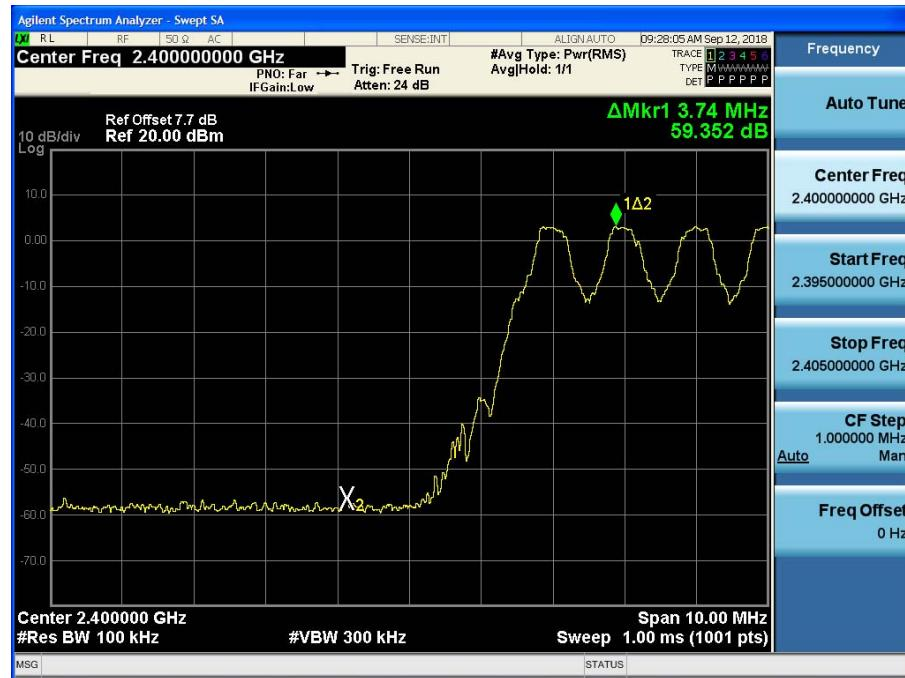
Test Plots with hopping (GFSK)
