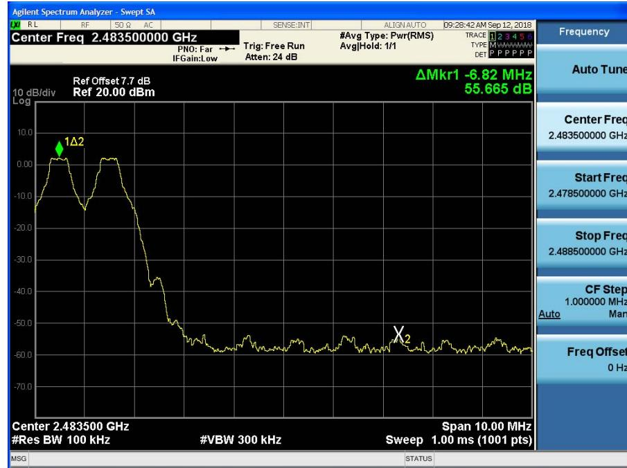
Test Plots with hopping (8DPSK)
