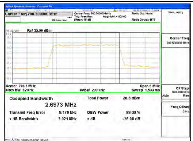
B12 / 3MHz / 64QAM/ Low CH
