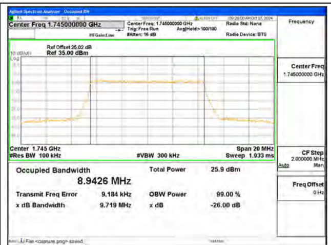
B66 / 10MHz / 16QAM/ Mid CH
