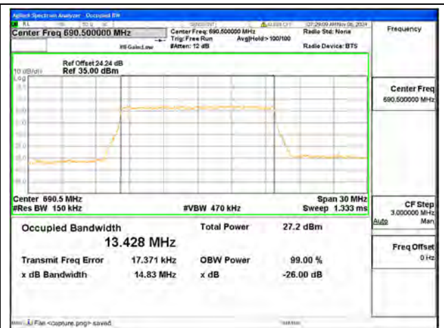
B71 / 15MHz / 16QAM/ High CH
