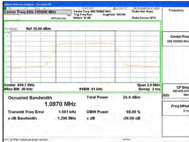
B12 / 1.4MHz / 64QAM/ Low CH
