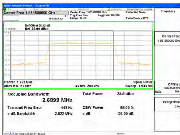
B2 / 3MHz / 16QAM/ Low CH
