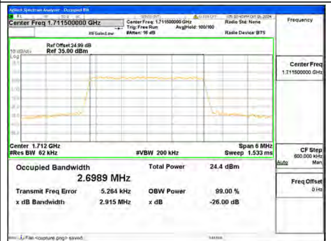
B4 / 3MHz / 64QAM/ Low CH
