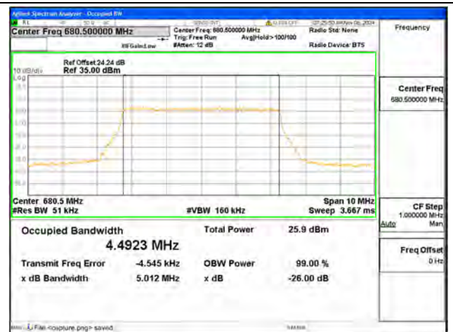
B71 / 5MHz / 64QAM/ Mid CH
