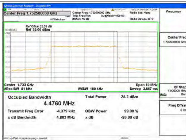
B4 / 5MHz / 16QAM/ Mid CH
