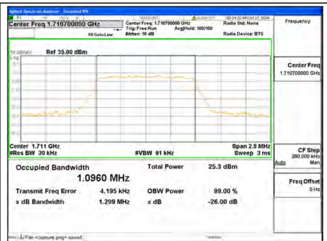
B66 / 1.4MHz / 16QAM/ Low CH
