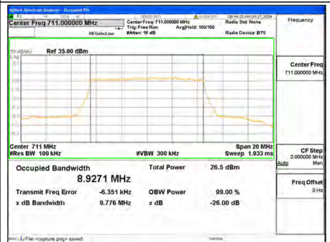
B17 / 10MHz / 64QAM/ High CH
