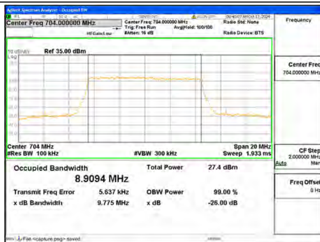
B12 / 10MHz / 16QAM/ Low CH
