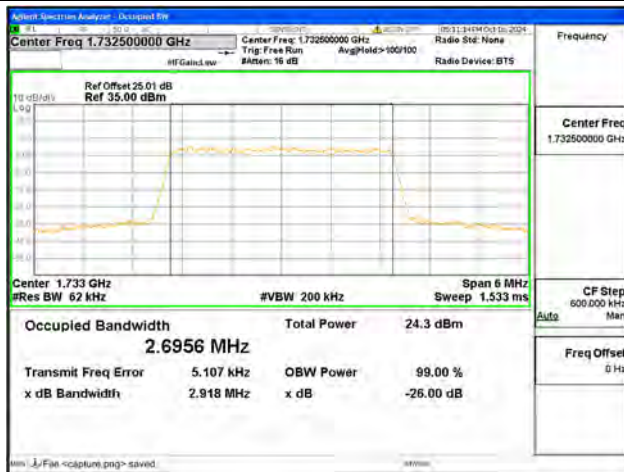
B4 / 3MHz / 64QAM/ Mid CH
