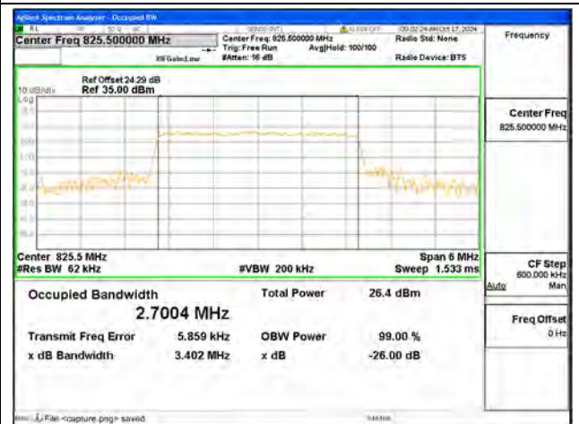
B5 / 3MHz / 64QAM/ Low CH
