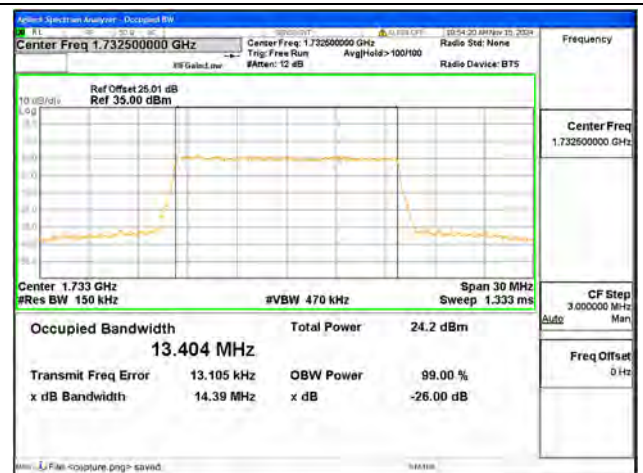
B4 / 15MHz / 64QAM/ Mid CH
