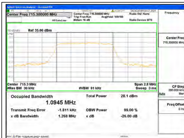
B12 / 1.4MHz / QPSK/ High CH
