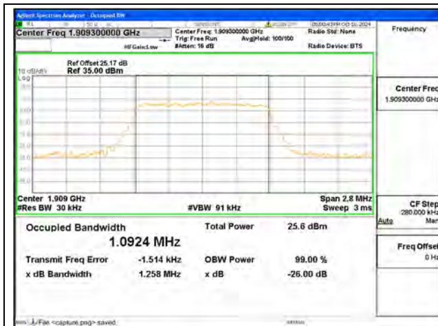
B2 / 1.4MHz / QPSK/ High CH
