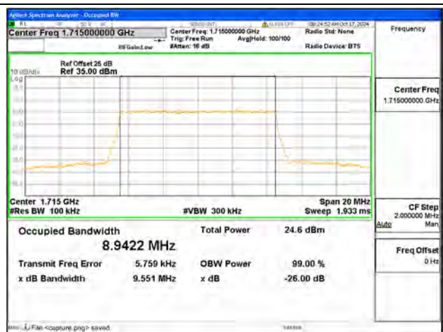
B4 / 10MHz / 64QAM/ Low CH
