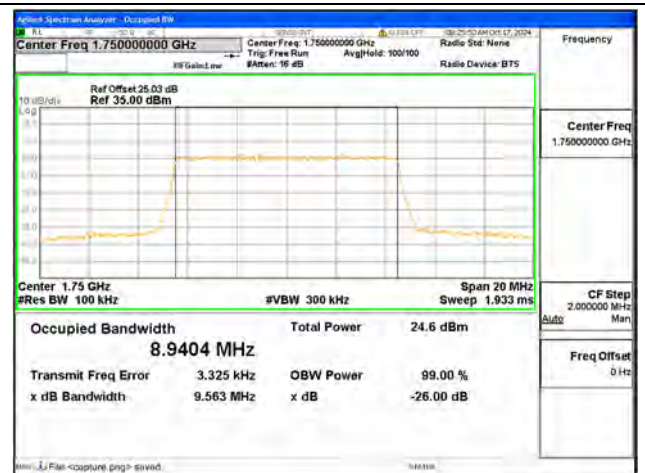
B4 / 10MHz / 64QAM/ High CH
