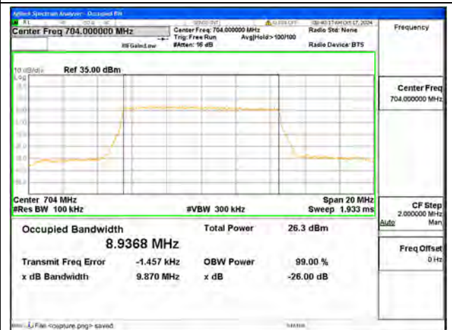
B12 / 10MHz / 64QAM/ Low CH
