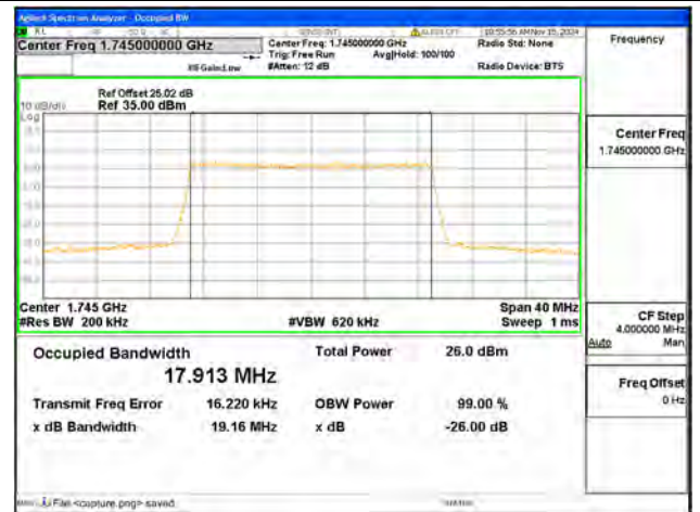
B4 / 20MHz / QPSK/ High CH
