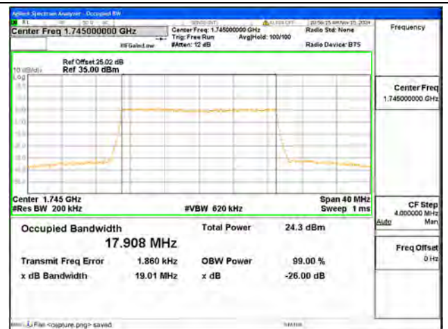
B4 / 20MHz / 64QAM/ High CH
