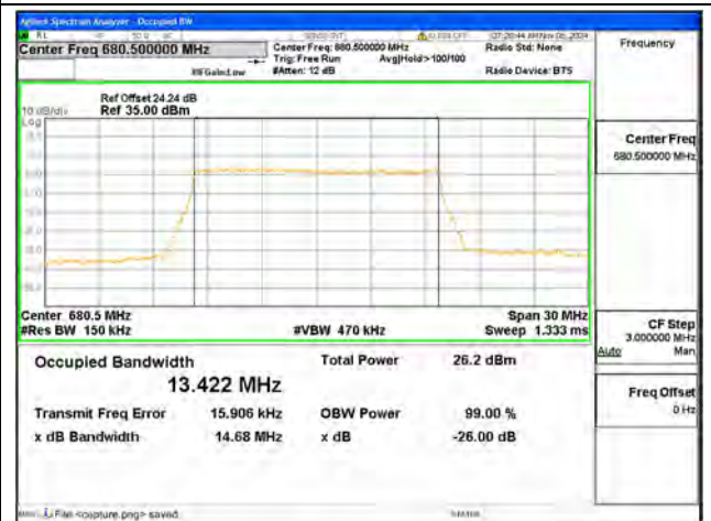
B71 / 15MHz / 64QAM/ Mid CH
