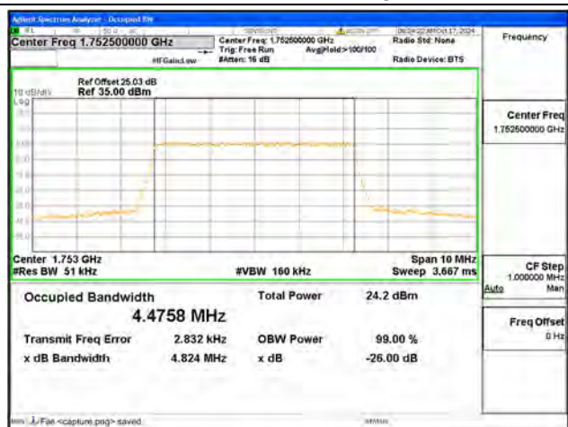
B4 / 5MHz / 64QAM/ High CH
