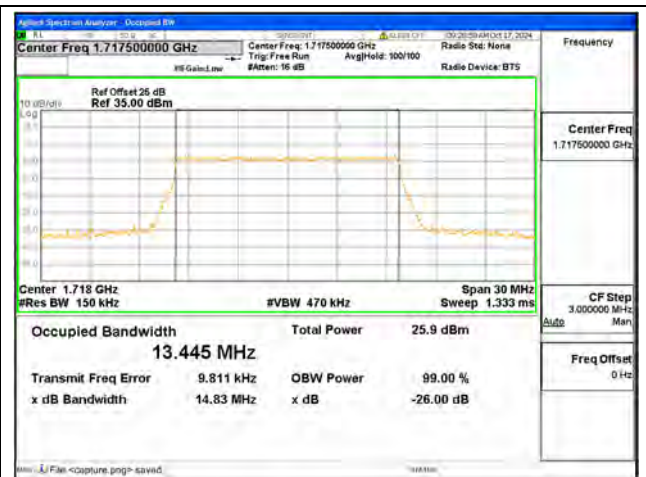
B66 / 15MHz / 16QAM/ Low CH
