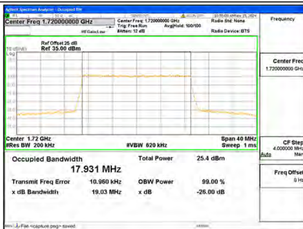
B4 / 20MHz / 16QAM/ Low CH
