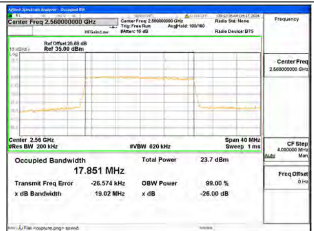
B7 / 20MHz / 64QAM/ High CH
