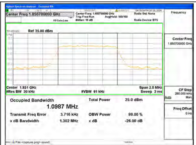
B2 / 1.4MHz / 16QAM/ Low CH
