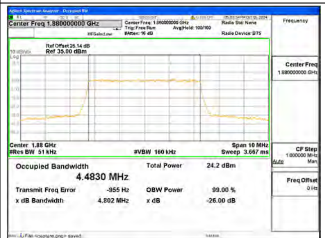
B2 / 5MHz / 64QAM/ Mid CH
