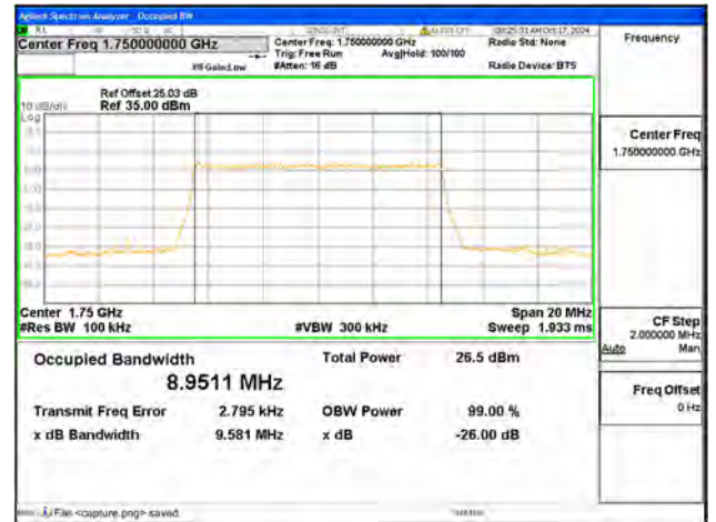
B4 / 10MHz / QPSK/ High CH
