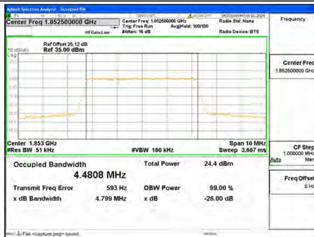
B2 / 5MHz / 64QAM/ Low CH
