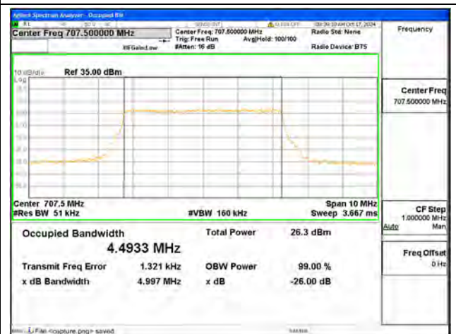
B12 / 5MHz / 64QAM/ Mid CH
