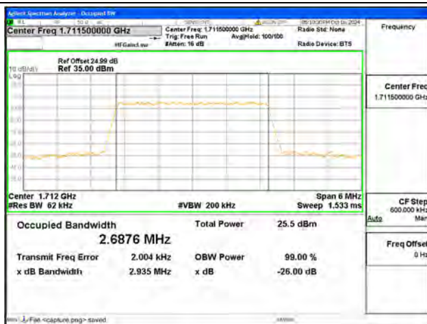
B4 / 3MHz / 16QAM/ Low CH
