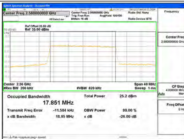
B7 / 20MHz / 16QAM/ High CH
