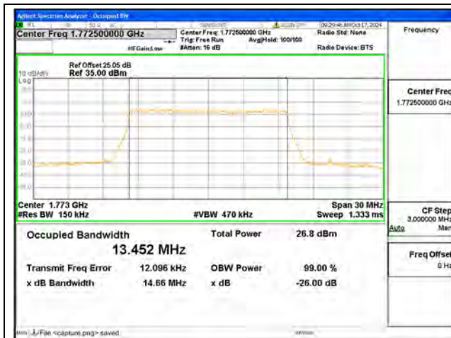
B66 / 15MHz / QPSK/ High CH
