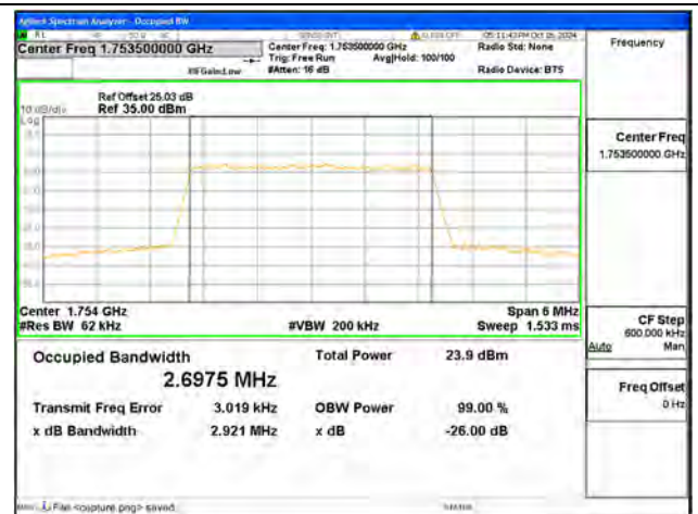
B4 / 3MHz / 64QAM/ High CH
