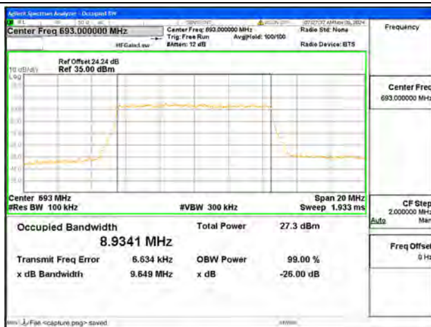
B71 / 10MHz / 16QAM/ High CH
