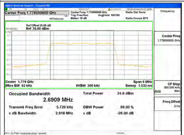
B66 / 3MHz / 64QAM/ High CH
