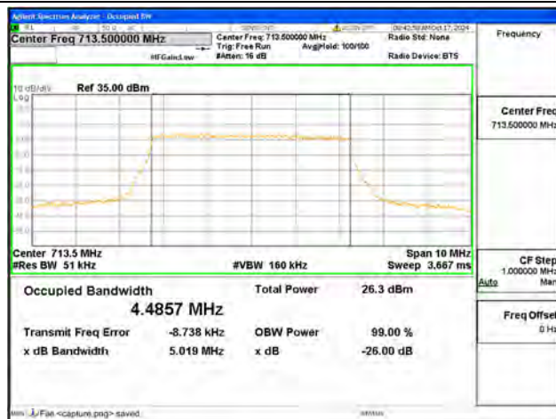
B17 / 5MHz / 64QAM/ High CH
