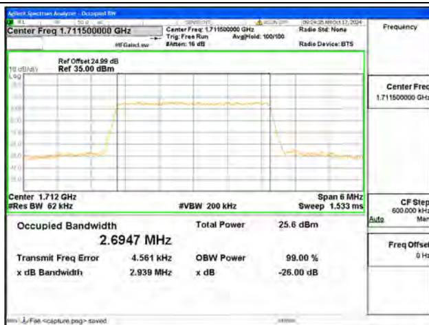
B66 / 3MHz / 16QAM/ Low CH
