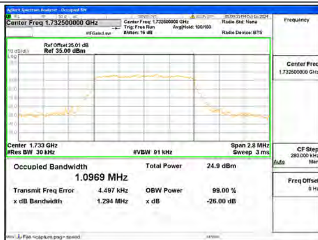
B4 / 1.4MHz / 16QAM/ Mid CH
