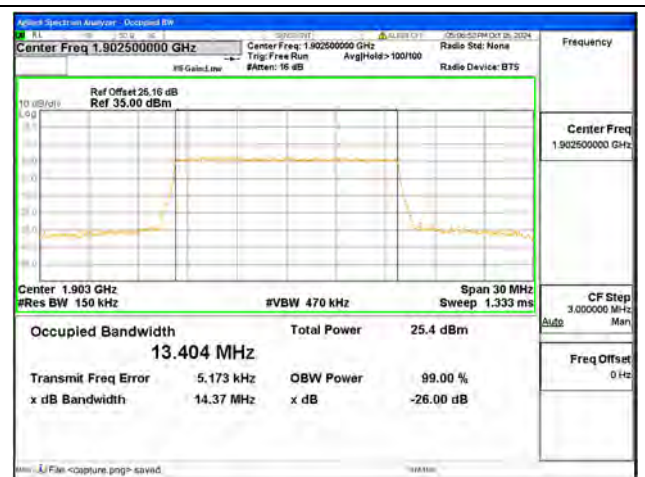
B2 / 15MHz / 16QAM/ High CH
