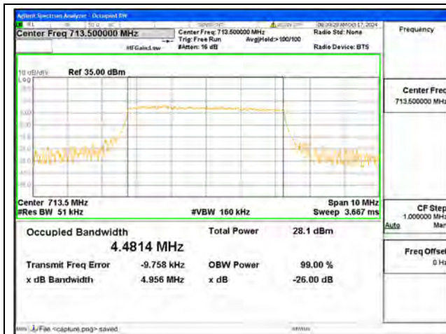
B12 / 5MHz / QPSK/ High CH
