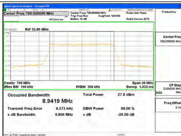
B17 / 10MHz / 16QAM/ Low CH
