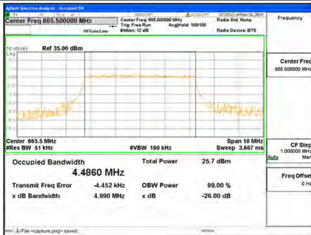
B71 / 5MHz / 64QAM/ Low CH
