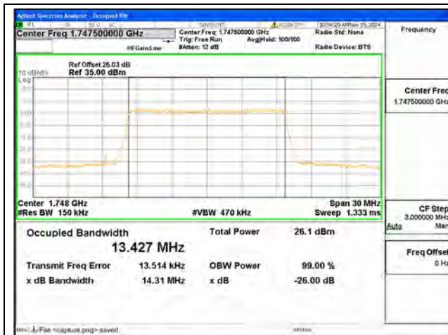
B4 / 15MHz / QPSK/ High CH
