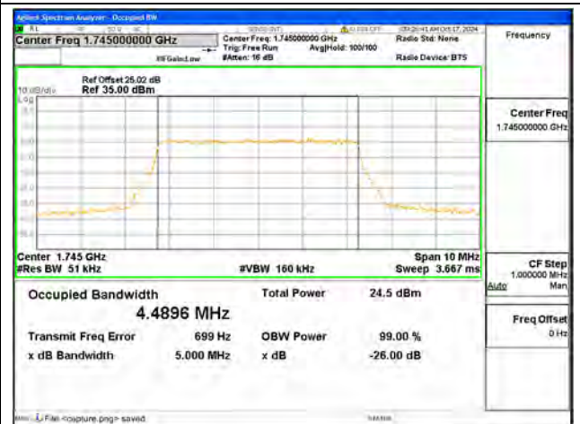
B66 / 5MHz / 64QAM/ Mid CH
