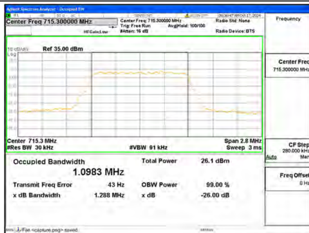
B12 / 1.4MHz / 64QAM/ High CH
