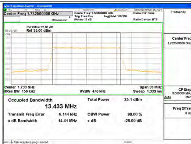
B4 / 15MHz / 16QAM/ Mid CH
