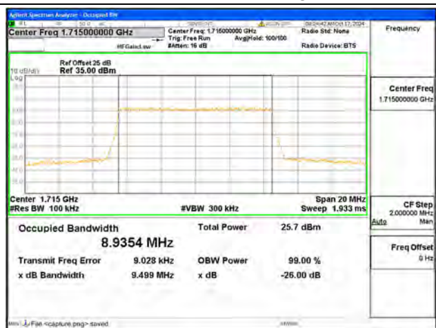
B4 / 10MHz / 16QAM/ Low CH
