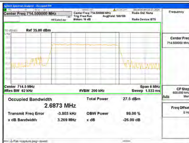
B12 / 3MHz / 16QAM/ High CH
