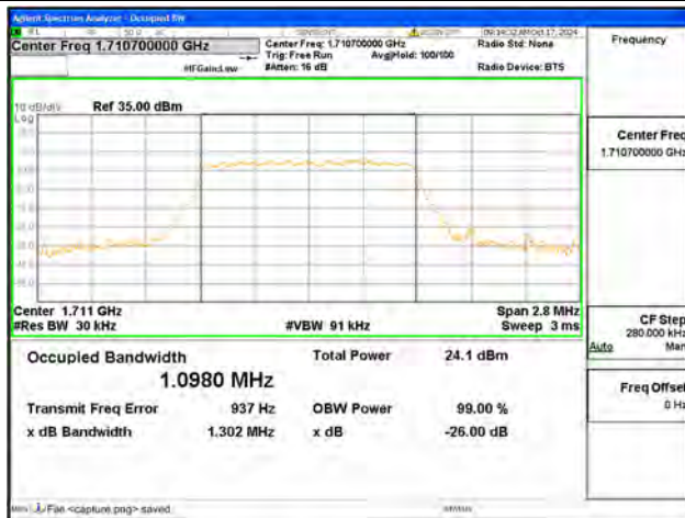
B66 / 1.4MHz / 64QAM/ Low CH
