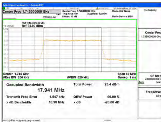
B4 / 20MHz / 16QAM/ High CH
