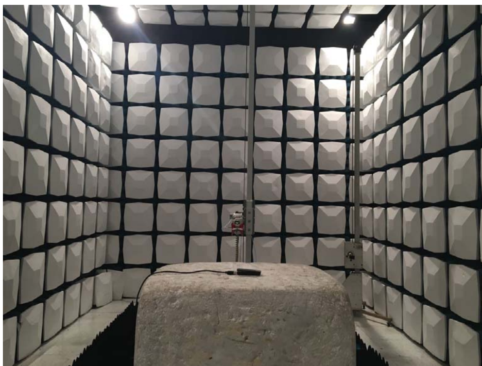
Description: Radiated Emission Test Setup for 1~18GHz
