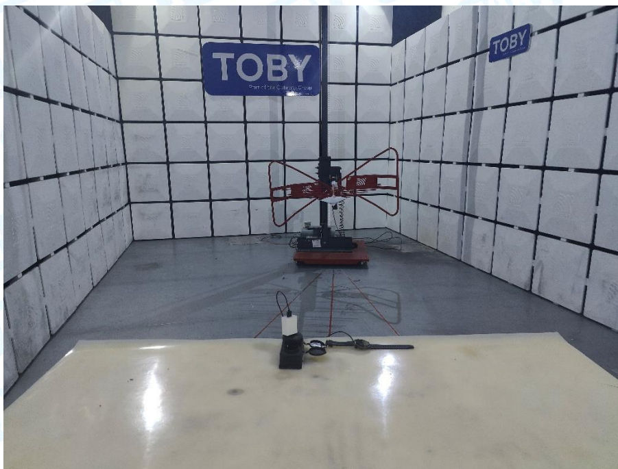
Photo of Setup for Radiated Emission (30MHz~1GHz)
