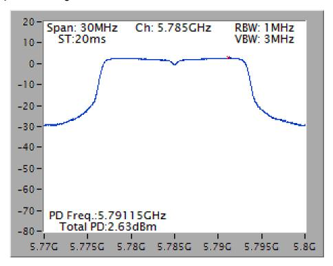
Power Density Plot on Configuration IEEE 802.11ac MCS0/Nss2 VHT20 / Chain 1 + Chain 2 / 5825 MHz
