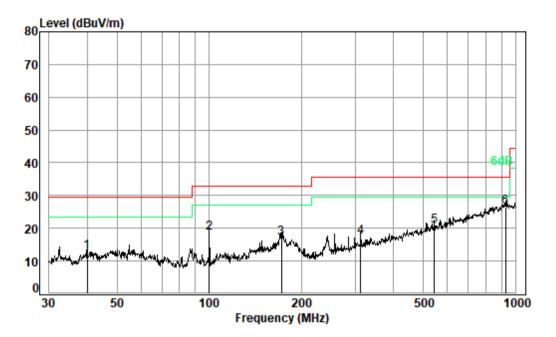
Condition: 10m HORIZONTAL Job No. : 03545AT Test Mode: 02
