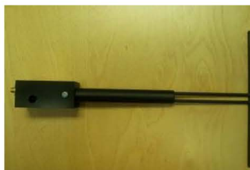
Figure 1 – MVG COMOSAR Validation Dipole
