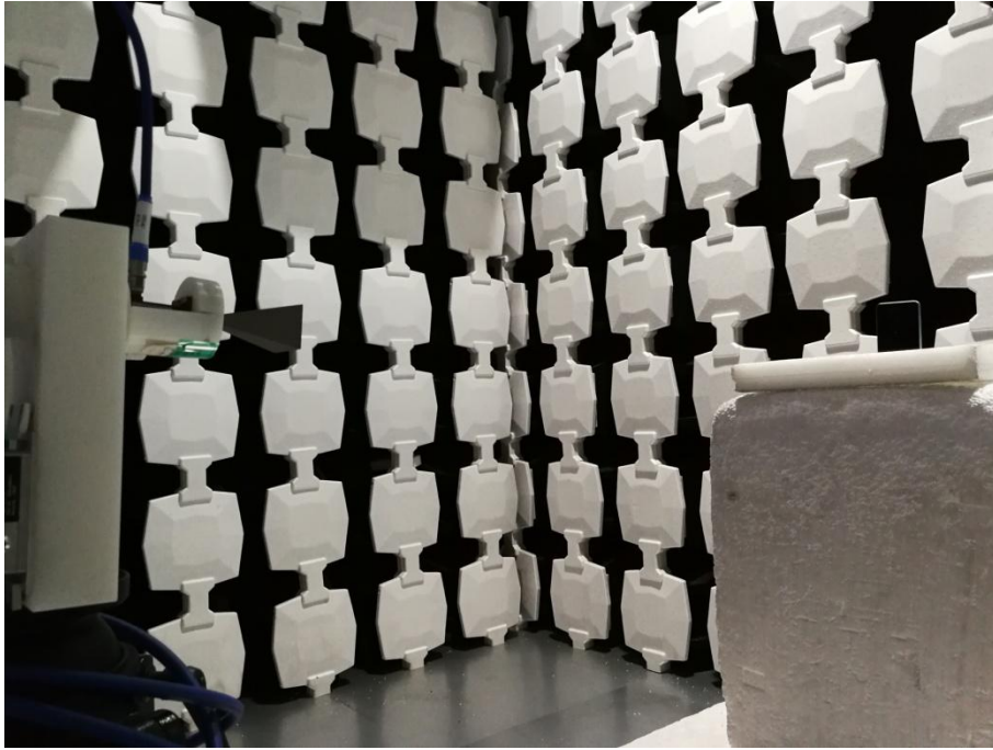
Description: Radiated Emission Test Setup (Above 18GHz)
