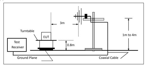
(c) For radiated emissions above 1000MHz
