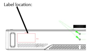
The label is attached to the bottom of the device with a permanent adhesive.
