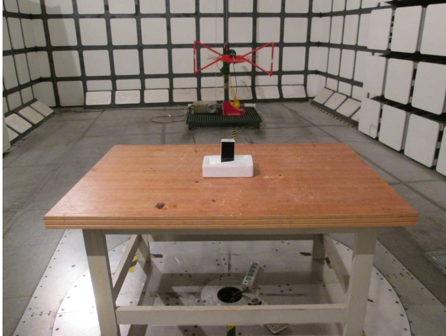
Radiated Emissions View (Below 1 GHz)
