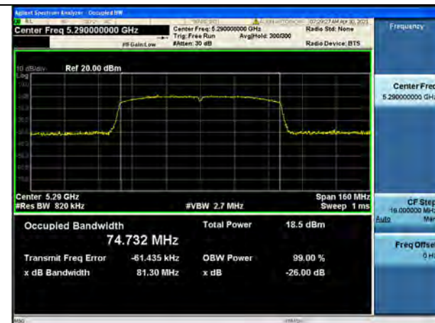
802.11ac_VHT80 UNII 3 BAND 26dB Bandwidth (CH 155)
