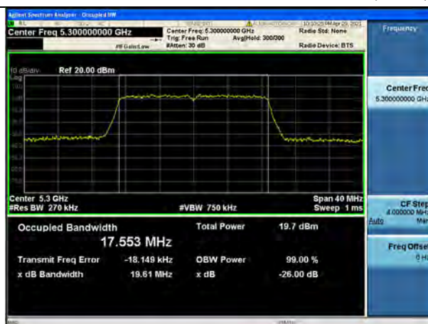
802.11n_HT20 UNII 3 BAND 26dB Bandwidth(CH 157)
