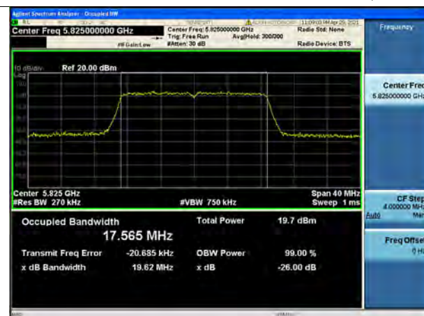
802.11ac_VHT20 UNII 3 BAND 26dB Bandwidth(CH 165)
