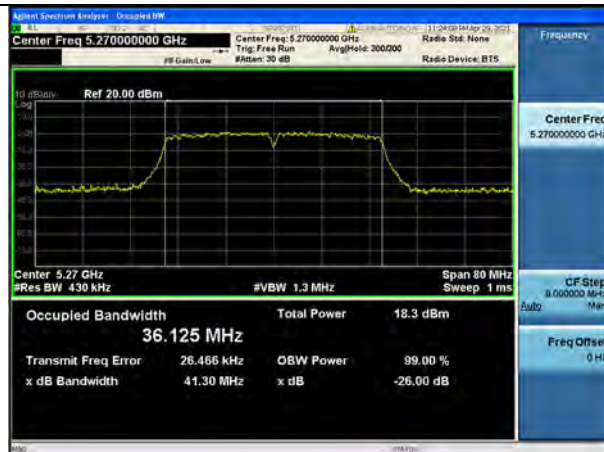
802.11n_HT40 UNII 3 BAND 26dB Bandwidth (CH 151)
