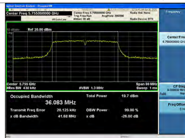
802.11ac_VHT40 UNII 3 BAND 26dB Bandwidth (CH 151)
