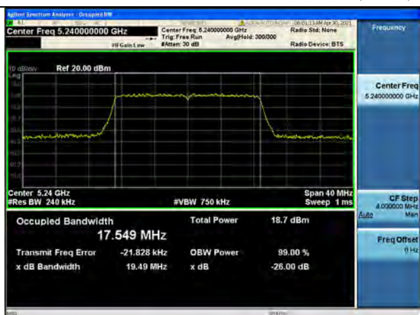
802.11n_HT20 UNII 2C BAND 26dB Bandwidth(CH 116)
