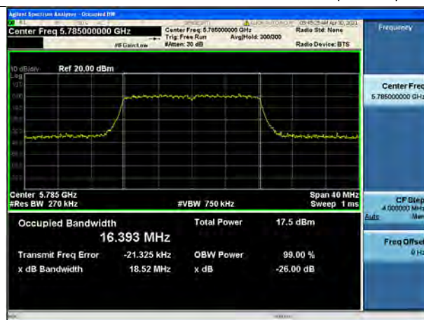
802.11a UNII 3 BAND 26dB Bandwidth (CH 157)
