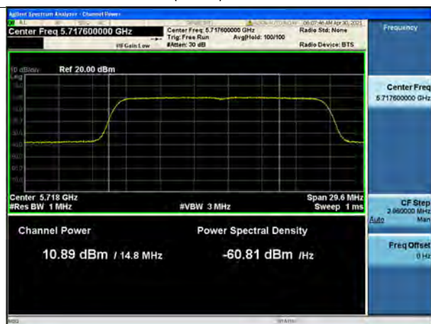
802.11ac(VHT20) UNII 2C Band
