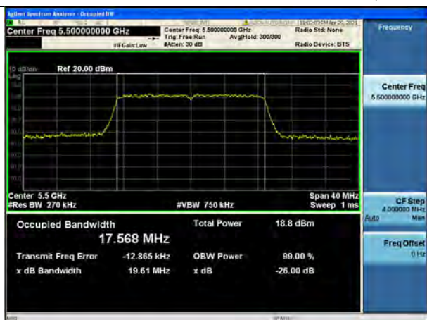
802.11ac_VHT20 UNII 2C BAND 26dB Bandwidth(CH 100)
