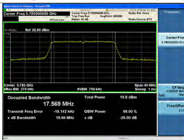
802.11n_HT20 UNII 3 BAND 26dB Bandwidth(CH 157)
