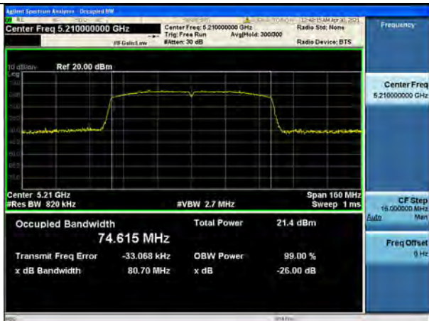
802.11ac_VHT80 UNII 2C BAND 26dB Bandwidth(CH 138)
