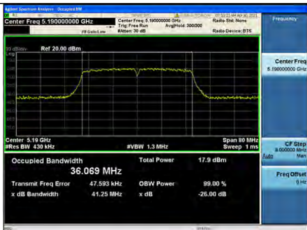
802.11ac_VHT40 UNII 2C BAND 26dB Bandwidth(CH 102)
