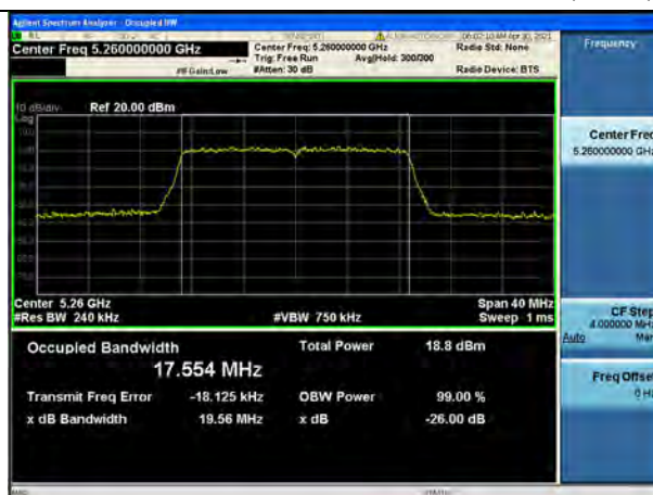
802.11n_HT20 UNII 3 BAND 26dB Bandwidth(CH 157)
