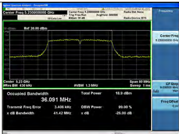
802.11ac_VHT40 UNII 2C BAND 26dB Bandwidth(CH 102)
