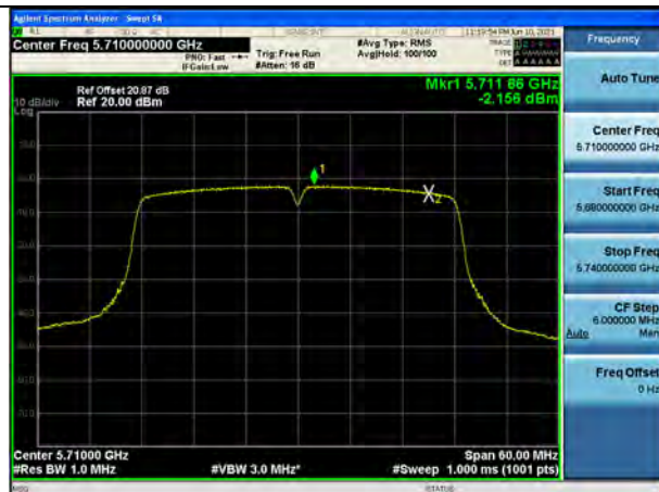
802.11ac(VHT40) UNII 2C Band
