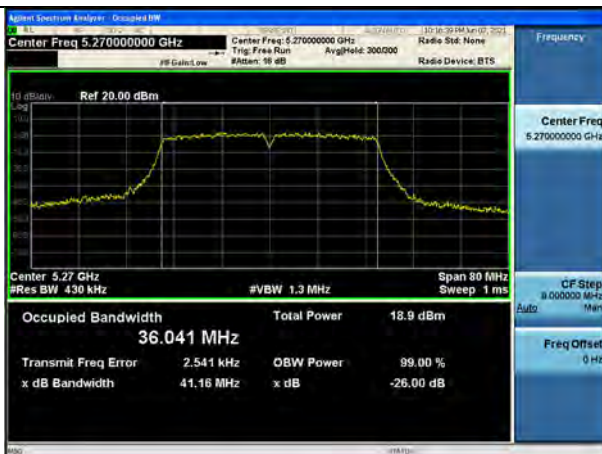
802.11n_HT40 UNII 3 BAND 26dB Bandwidth (CH 151)
