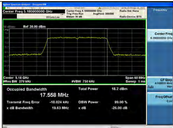
802.11ac_VHT20 UNII 2C BAND 26dB Bandwidth(CH 100)
