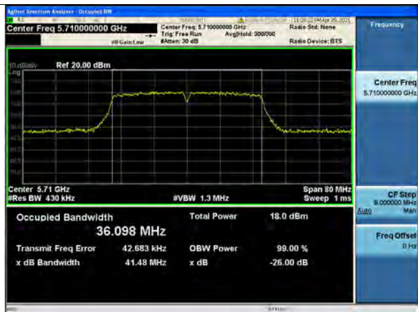
802.11n_HT40 UNII 2C BAND 26dB Bandwidth(CH 142)
