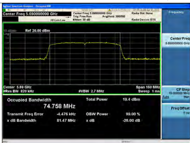
802.11ac_VHT80 UNII 2C BAND 26dB Bandwidth(CH 138)
