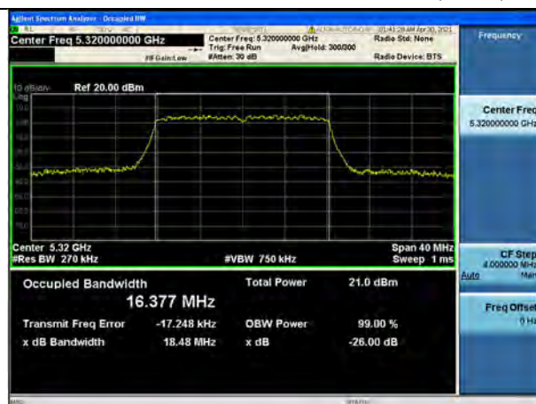
802.11a UNII 3 BAND 26dB Bandwidth (CH 157)
