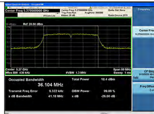
802.11ac_VHT40 UNII 3 BAND 26dB Bandwidth (CH 151)
