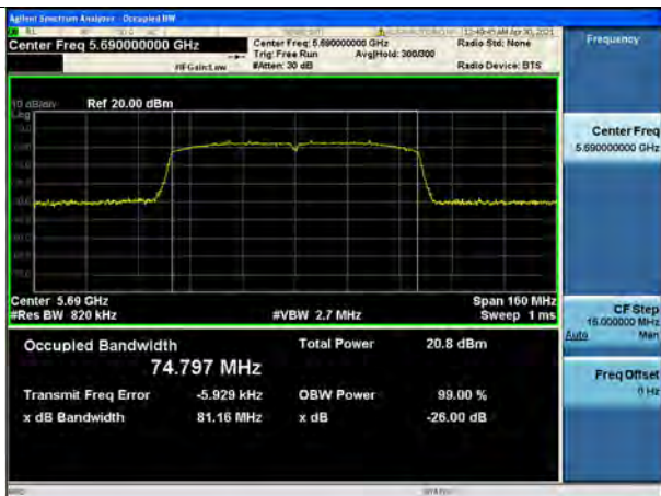
802.11ac_VHT80 UNII 2C BAND 26dB Bandwidth(CH 138)
