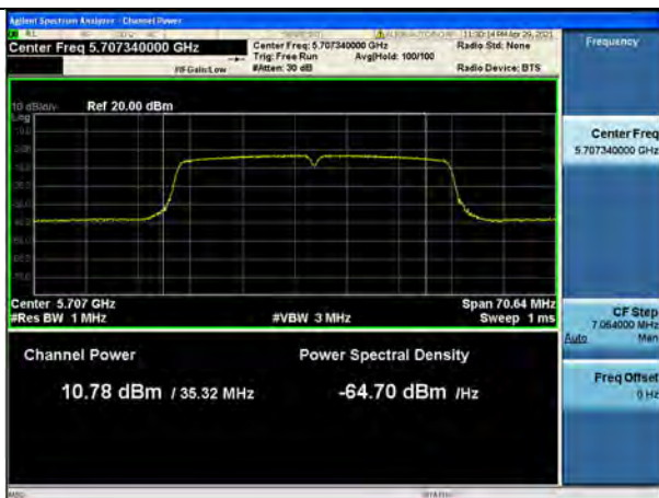
802.11ac(VHT40) UNII 2C Band
