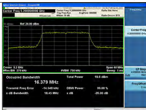
802.11a UNII 2C BAND 26dB Bandwidth (CH 144)
