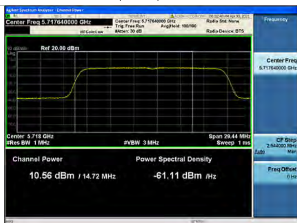
802.11ac(VHT20) UNII 2C Band
