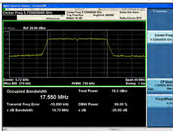
802.11n_HT20 UNII 2C BAND 26dB Bandwidth(CH 144)
