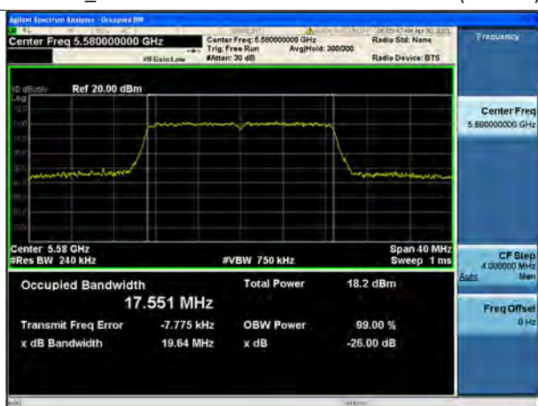
802.11n_HT20 UNII 2C BAND 26dB Bandwidth(CH 116)
