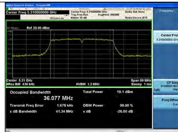
802.11ac_VHT40 UNII 3 BAND 26dB Bandwidth (CH 151)
