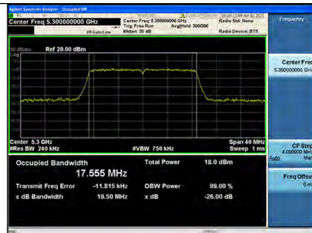
802.11ac_VHT20 UNII 3 BAND 26dB Bandwidth(CH 157)
