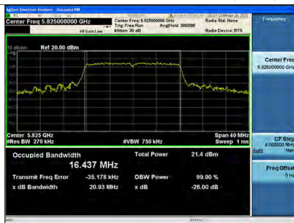
802.11a UNII 3 BAND 26dB Bandwidth (CH 165)
