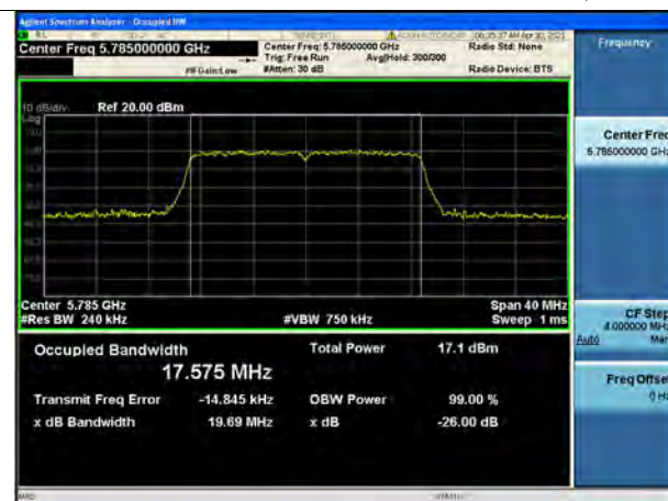
802.11ac_VHT20 UNII 3 BAND 26dB Bandwidth(CH 157)
