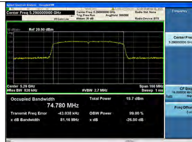
802.11ac_VHT80 UNII 3 BAND 26dB Bandwidth (CH 155)
