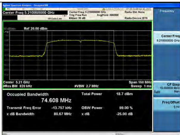
802.11ac_VHT80 UNII 2C BAND 26dB Bandwidth(CH 138)
