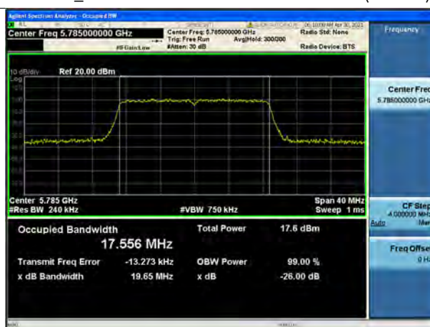
802.11n_HT20 UNII 3 BAND 26dB Bandwidth(CH 157)
