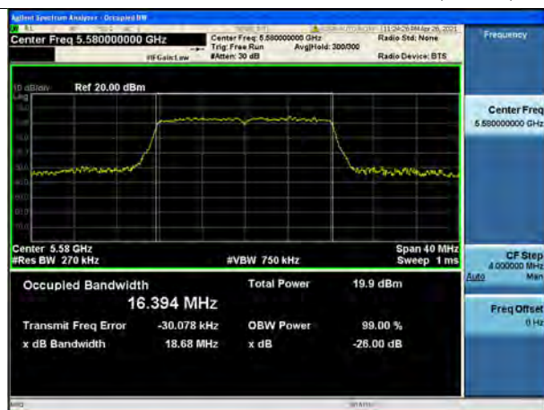
802.11a UNII 2C BAND 26dB Bandwidth (CH116)
