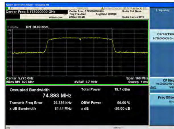
802.11ac_VHT80 UNII 3 BAND 26dB Bandwidth (CH 155)
