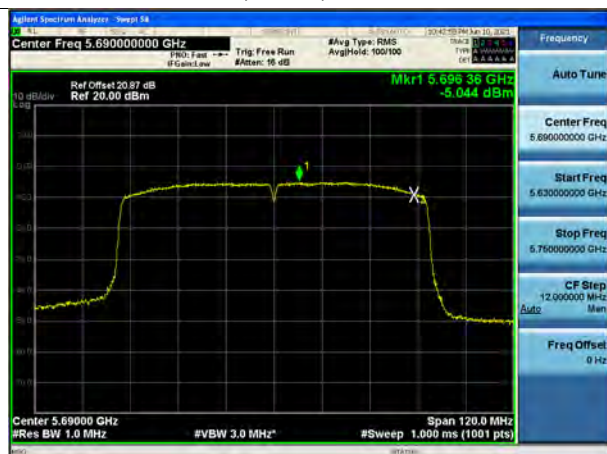
802.11ac(VHT80) UNII 2C Band
