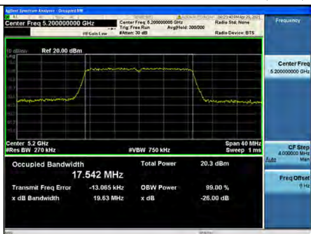
802.11n_HT20 UNII 2C BAND 26dB Bandwidth(CH 144)
