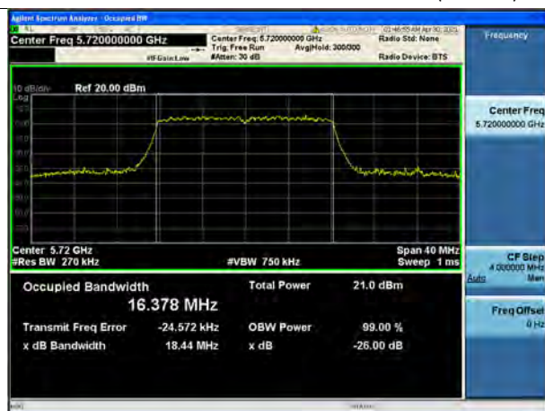
802.11a UNII 2C BAND 26dB Bandwidth (CH 144)
