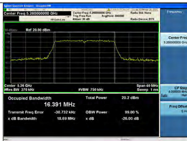
802.11a UNII 3 BAND 26dB Bandwidth (CH 165)
