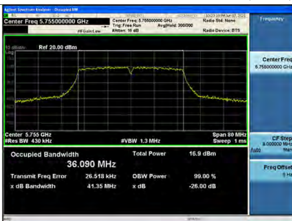
802.11n_HT40 UNII 3 BAND 26dB Bandwidth (CH 151)
