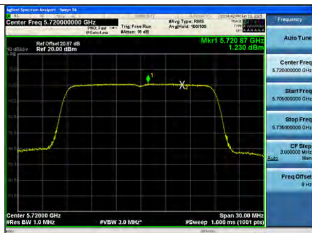
802.11ac(VHT20) UNII 2C Band
