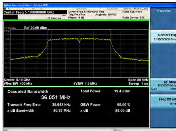
802.11n_HT40 UNII 2C BAND 26dB Bandwidth(CH 102)
