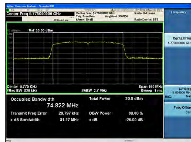
802.11ac_VHT80 UNII 3 BAND 26dB Bandwidth (CH 155)
