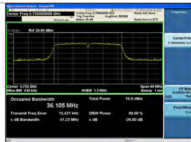
802.11ac_VHT40 UNII 3 BAND 26dB Bandwidth (CH 151)
