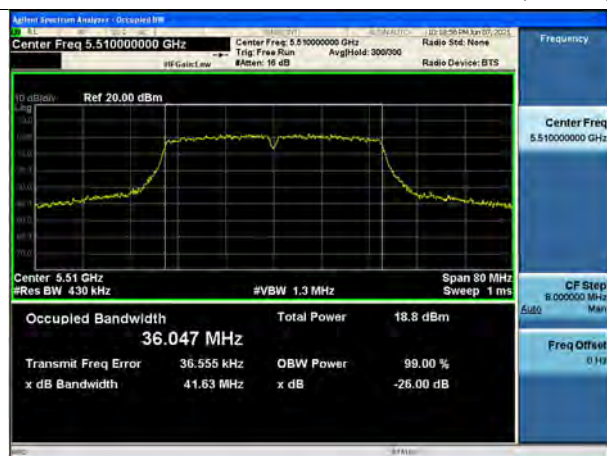
802.11n_HT40 UNII 2C BAND 26dB Bandwidth(CH 102)
