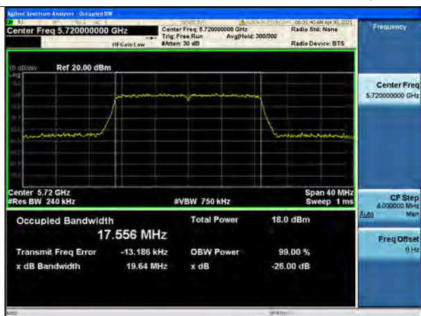
802.11ac_VHT20 UNII 2C BAND 26dB Bandwidth(CH 144)
