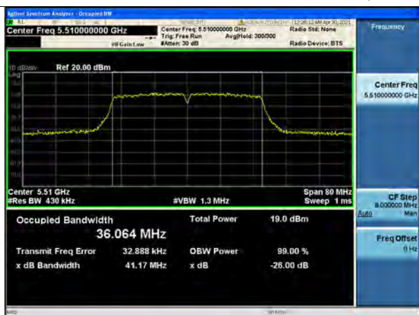
802.11ac_VHT40 UNII 2C BAND 26dB Bandwidth(CH 102)
