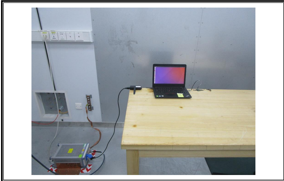
RADIATED RF MEASUREMENT SETUP (30MHz ~ 1 GHz)
