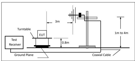
(c) For radiated emissions above 1000MHz
