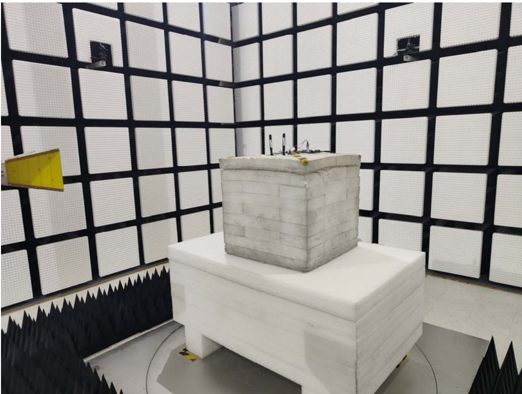
Radiated Emissions Above 1G View Whip ANT
