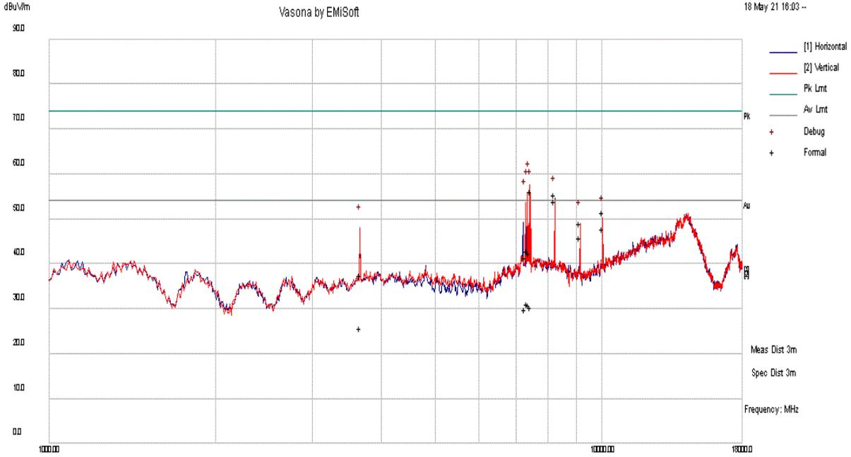
Radiated Emissions Template: FCC 15.209 (3m) 1-18GHz
