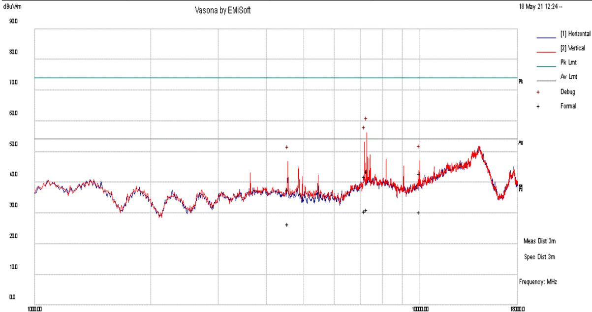
Radiated Emissions Template: FCC 15.209 (3m) 1-18GHz
