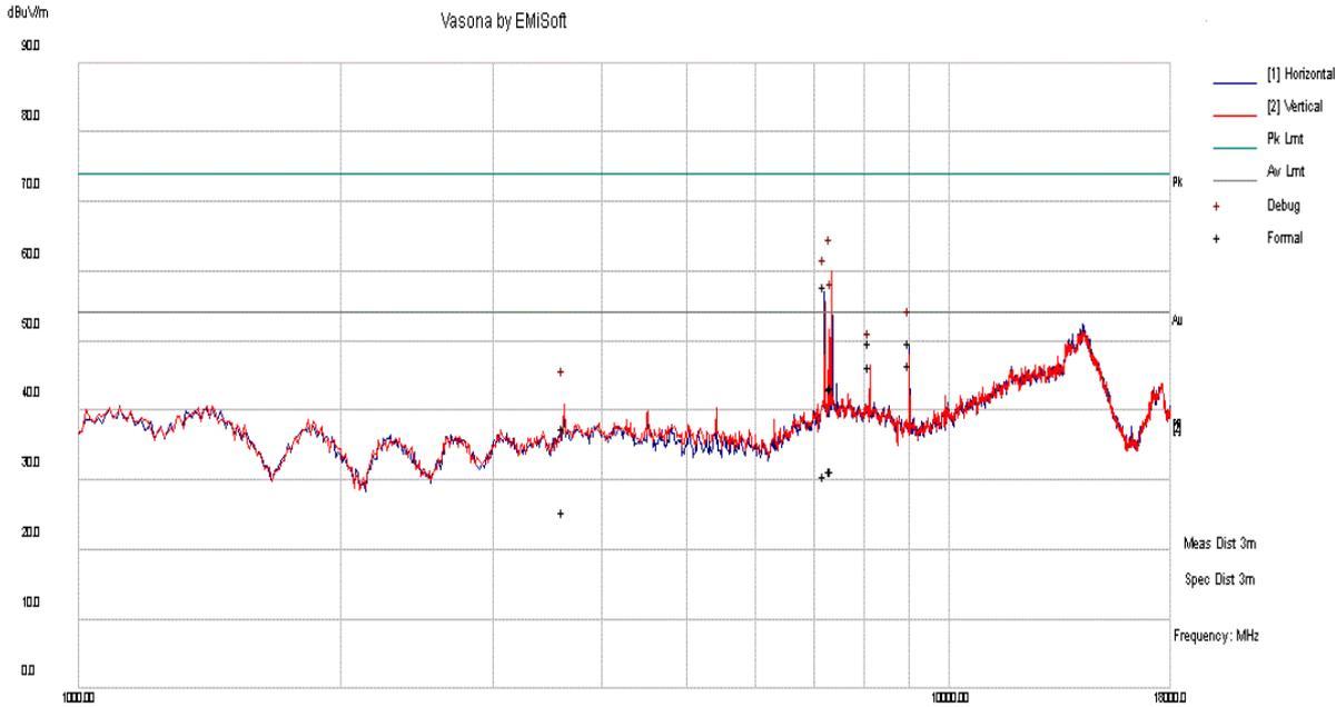
Radiated Emissions Template: FCC 15.209 (3m) 1-18GHz
