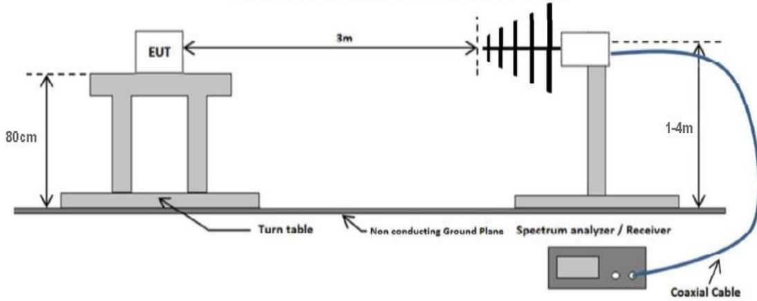
**Radiated emissions test setup above 1 GHz**
