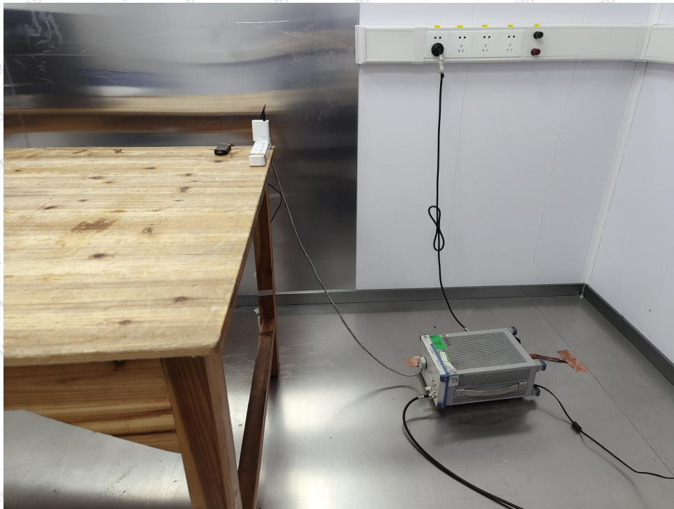
Photo of Conducted Emission Measurement
