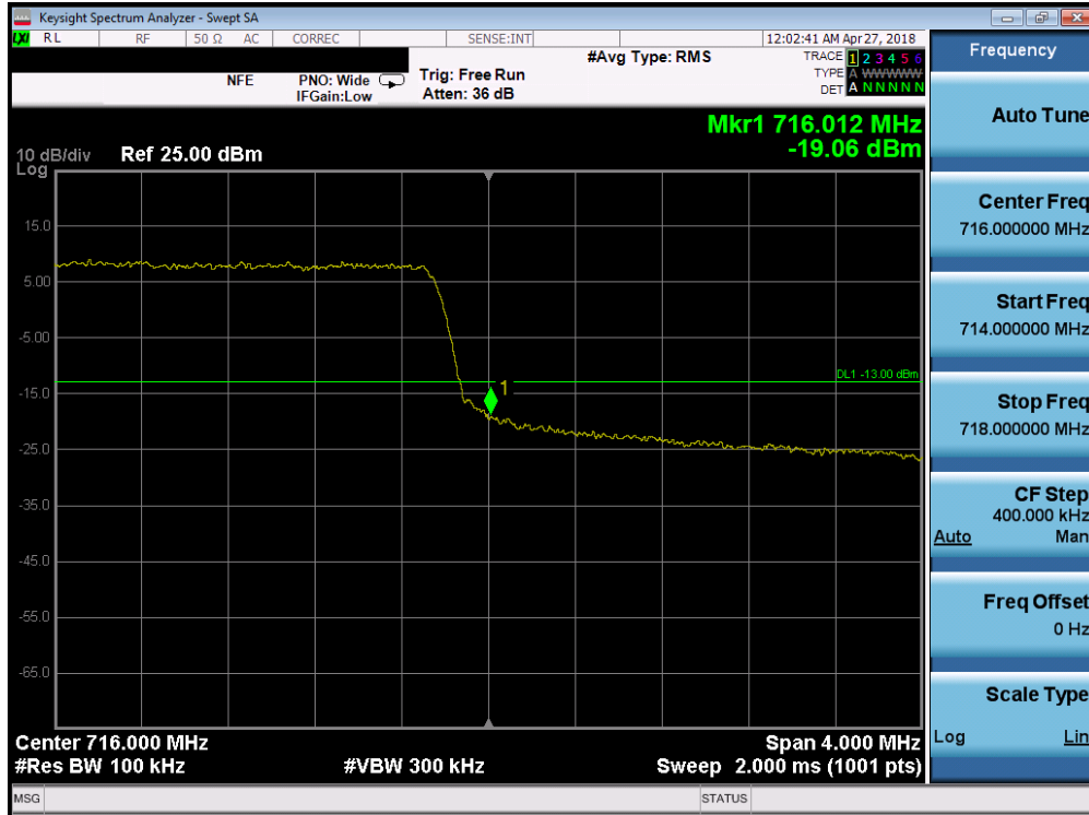
Plot 7-138. Upper Band Edge Plot (Band 12/17 - 5.0MHz QPSK - Full RB Configuration)
