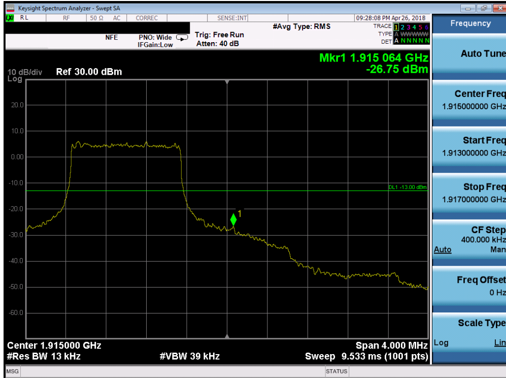
Plot 7-202. Upper Band Edge Plot (Band 25 - 1.4MHz QPSK - Full RB Configuration)
