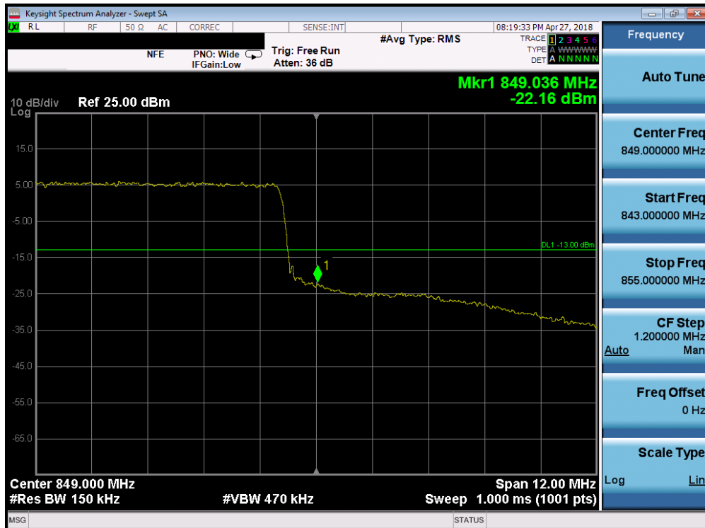
Plot 7-161. Upper Band Edge Plot (Band 26 - 15.0MHz QPSK - Full RB Configuration)
