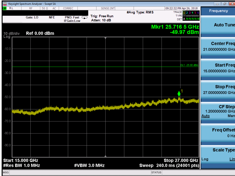
Plot 7-129. Conducted Spurious Plot (Band 41 - 20.0MHz QPSK - RB Size 1, RB Offset 0 - High Channel)
