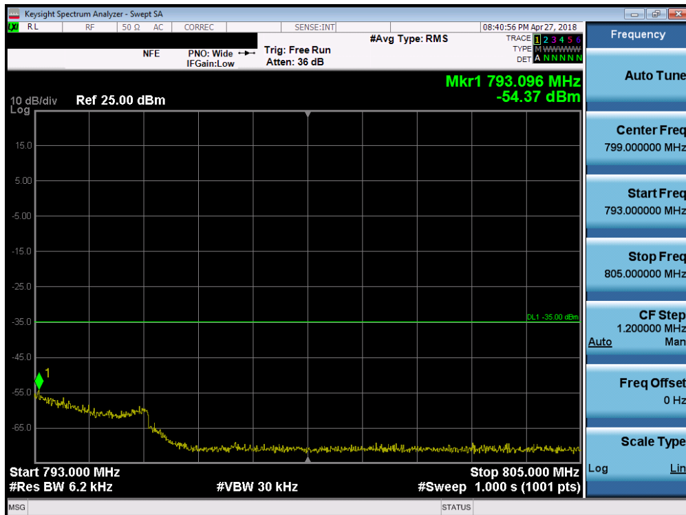
Plot 7-149. Upper Emission Mask Band Edge Plot (Band 13 - 10.0MHz QPSK - Full RB Configuration)
