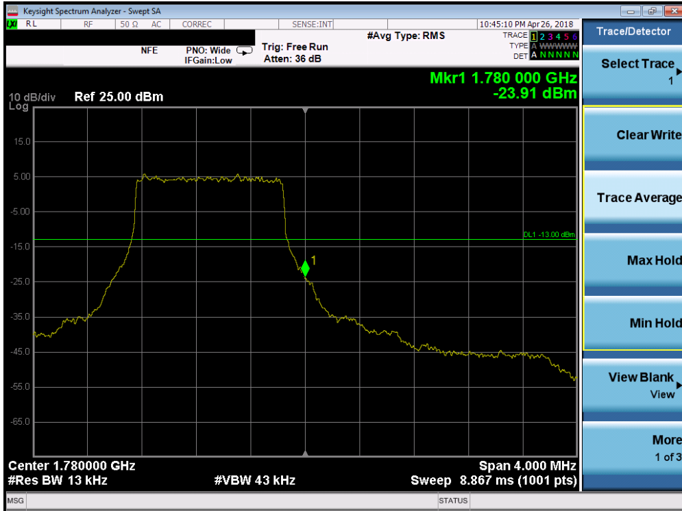
Plot 7-166. Upper Band Edge Plot (Band 66 - 1.4MHz QPSK - Full RB Configuration)
