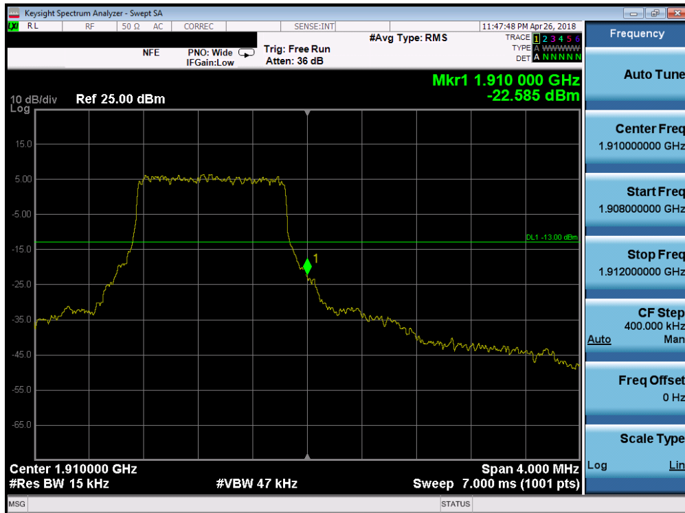
Plot 7-200. Upper Band Edge Plot (Band 2 - 1.4MHz QPSK - Full RB Configuration)
