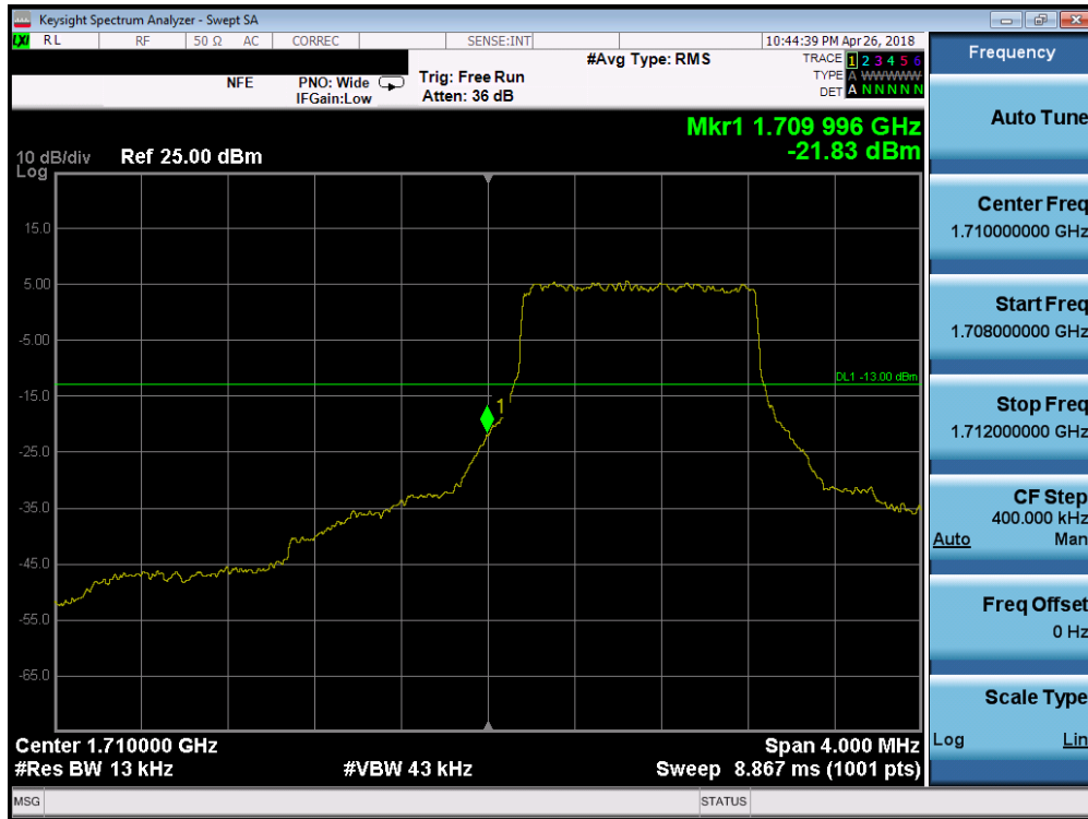
Plot 7-162. Lower Band Edge Plot (Band 66/4 - 1.4MHz QPSK - Full RB Configuration)
