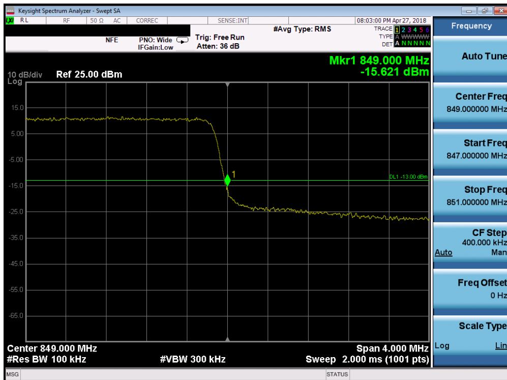
Plot 7-155. Upper Band Edge Plot (Band 26/5 - 3.0MHz QPSK - Full RB Configuration)
