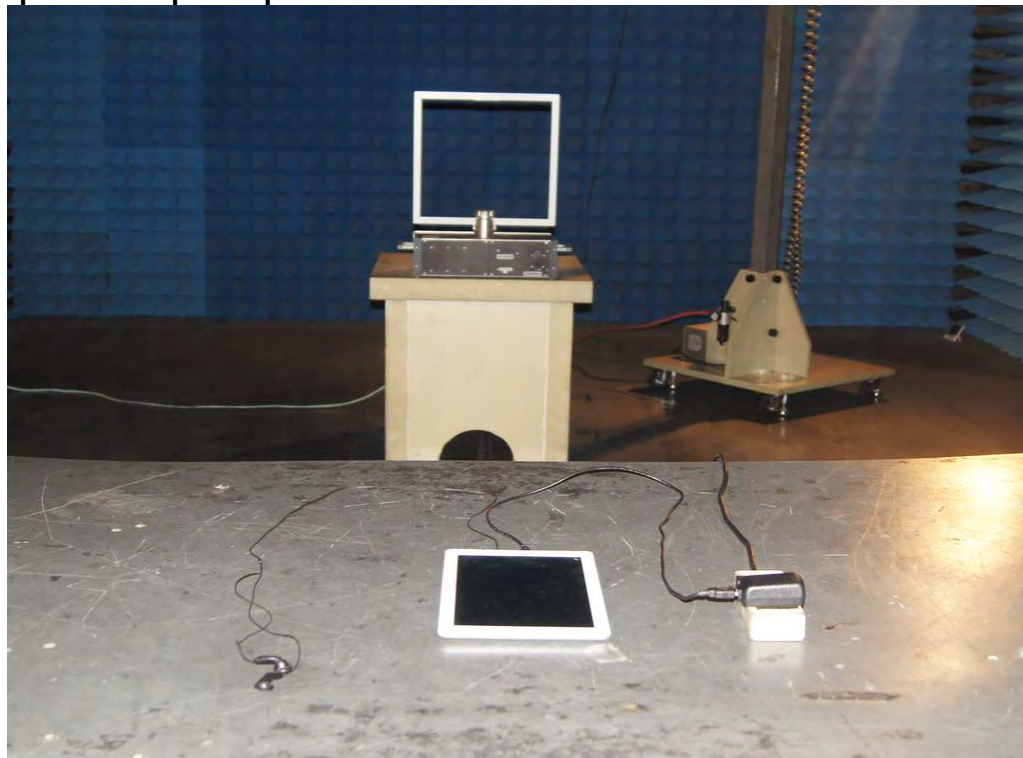
Photograph 2: Set-up for Spurious Emissions below 30MHz
