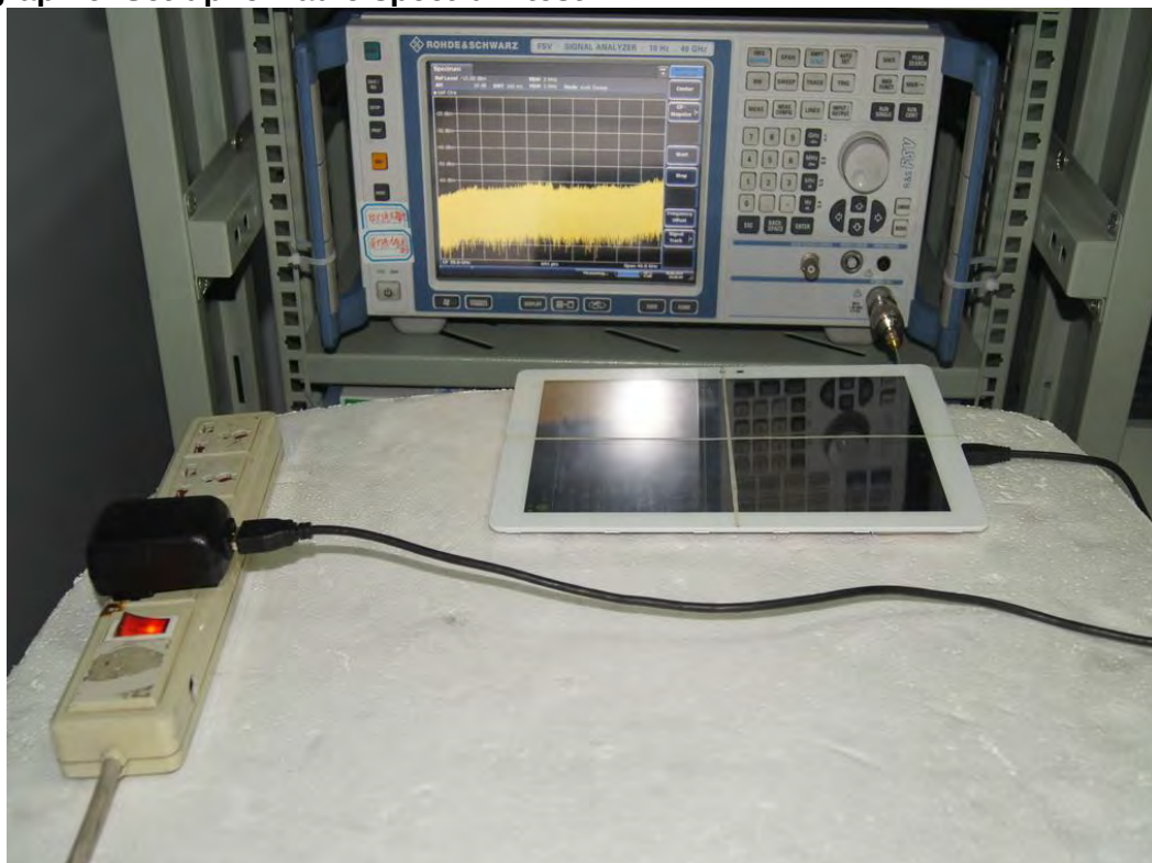
Photograph 6: Set-up for radio spectrum test
