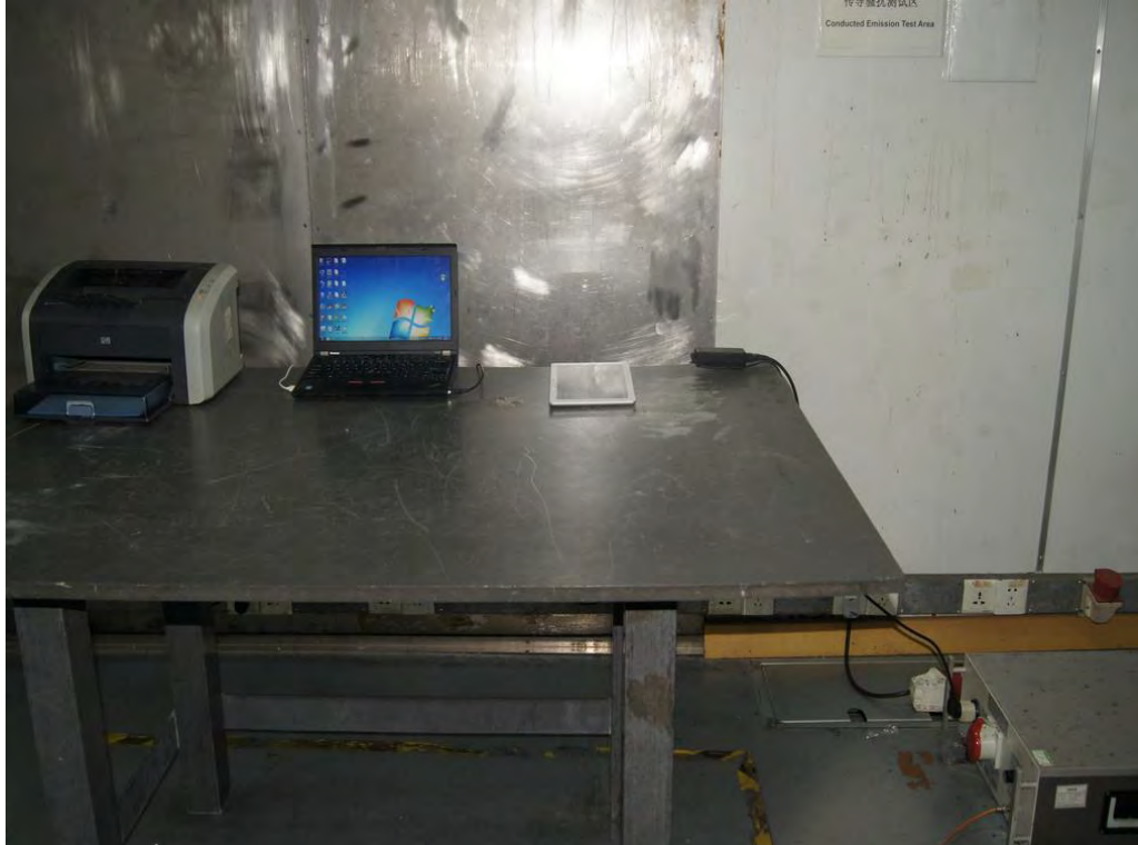
Photograph 2: Set-up for Spurious Emissions below 30MHz
