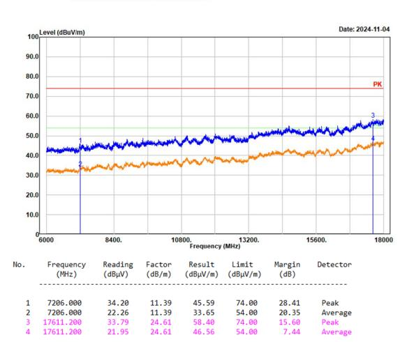
Project No.: 2403Y36748E-RF Tester: Mack Huang Polarization: vertical Note: BDR Low Channel 2402MHz Chain 1
