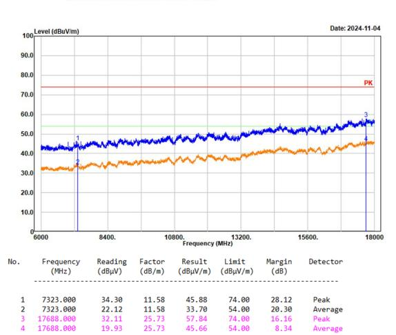
Project No.: 2403Y36748E-RF Tester: Mack Huang Polarization: vertical Note: 3EDR Middle Channel 2441MHz Chain 0
