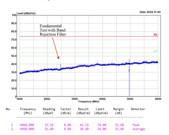
Project No.: 2403Y36748E-RF Tester: Mack Huang Polarization: vertical Note: BDR High Channel 2480MHz Chain 0
