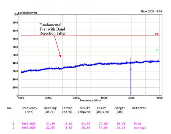
Project No.: 2403Y36748E-RF Tester: Mack Huang Polarization: vertical Note: 2EDR High Channel 2480MHz Chain 1
