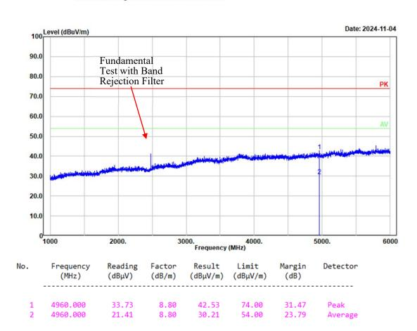
Project No.: 2403Y36748E-RF Tester: Mack Huang Polarization: horizontal Note: 2EDR High Channel 2480MHz Chain 1
