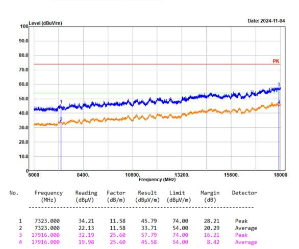
Project No.: 2403Y36748E-RF Tester: Mack Huang Polarization: horizontal Note: 3EDR Middle Channel 2441MHz Chain 0
