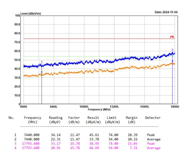
Project No.: 2403Y36748E-RF Tester: Mack Huang Polarization: horizontal Note: BDR High Channel 2480MHz Chain 0
