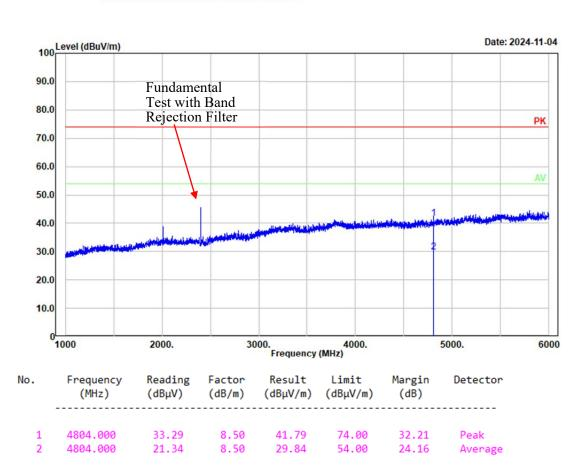
Project No.: 2403Y36748E-RF Tester: Mack Huang Polarization: vertical Note: BDR Low Channel 2402MHz Chain 1
