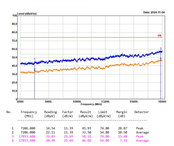
Project No.: 2403Y36748E-RF Tester: Mack Huang Polarization: horizontal Note: 2EDR Low Channel 2402MHz Chain 0
