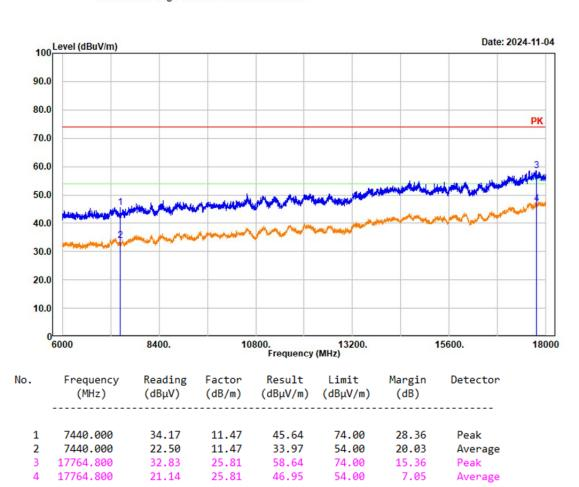
Project No.: 2403Y36748E-RF Tester: Mack Huang Polarization: vertical Note: 2EDR High Channel 2480MHz Chain 1
