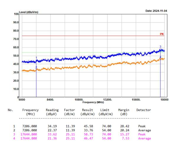
Project No.: 2403Y36748E-RF Tester: Mack Huang Polarization: horizontal Note: BDR Low Channel 2402MHz Chain 1
