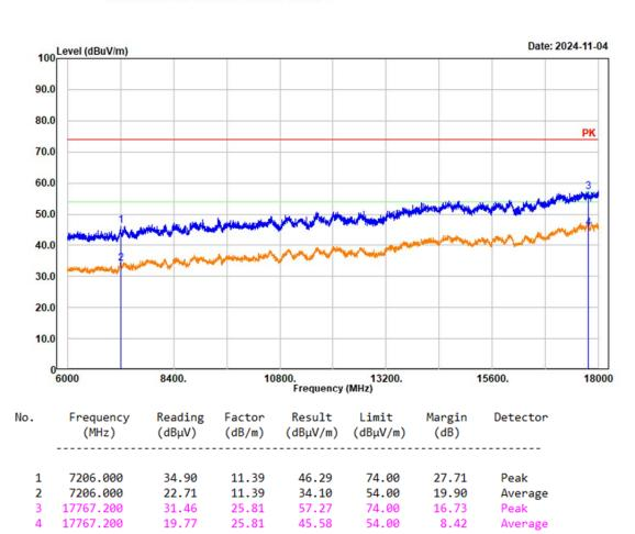
Project No.: 2403Y36748E-RF Tester: Mack Huang Polarization: vertical Note: 2EDR Low Channel 2402MHz Chain 0
