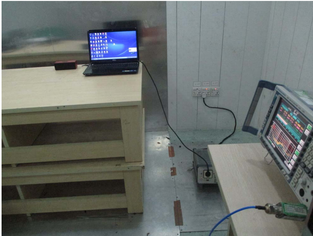
FCC RADIATED EMISSION TEST SETUP
