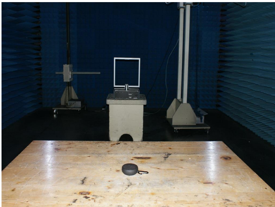
Photograph 2: Set-up for Radiated Spurious Emission, 9KHz - 30MHz
