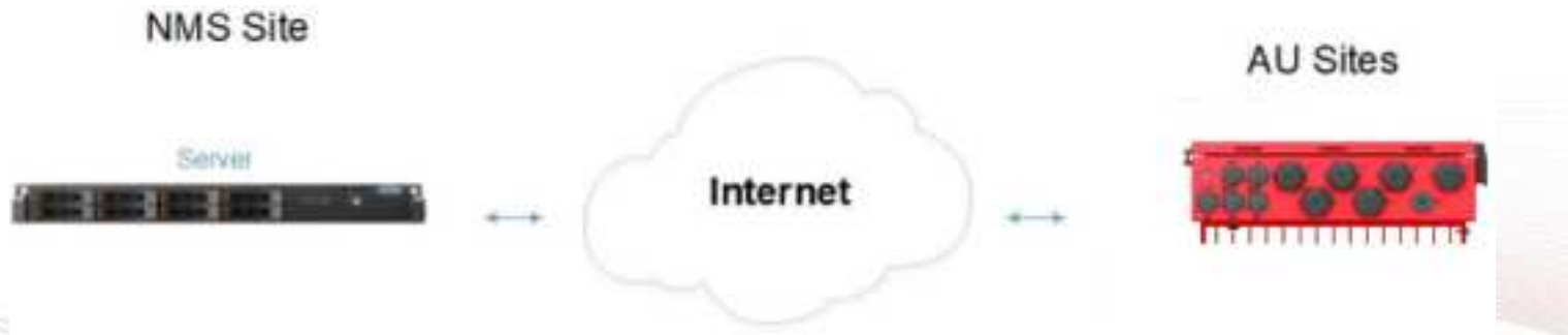
Figure 11. NMS System Architecture
