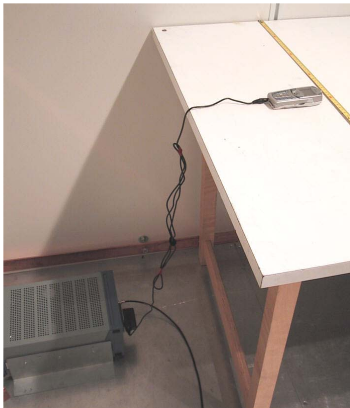
Picture 1: Conducted emission test setup
