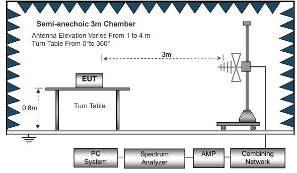
(C) Radiated Emission Test-Up Frequency Above 1GHz
