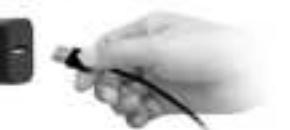
2. Insert the micro USB end of the power cable into the micro USB port on the wireless charger. The LED indicator will flash blue three times to indicate power connectivity.
