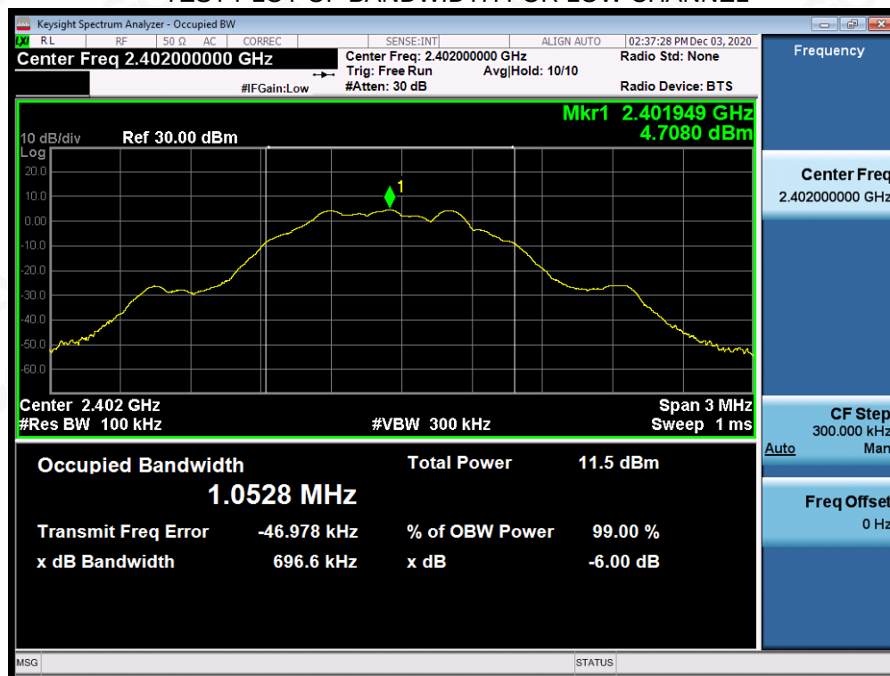
TEST PLOT OF BANDWIDTH FOR LOW CHANNEL
