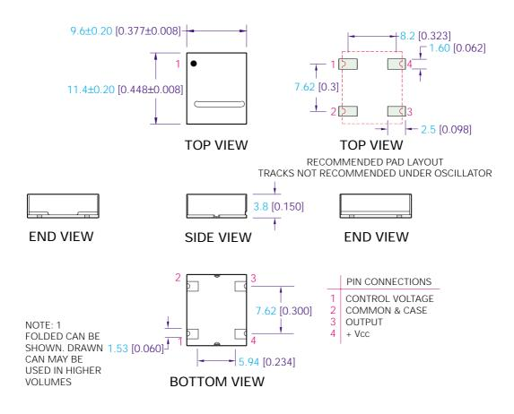
TITLE: VTXO200U MODEL FILENAME: CAT006 **REVISION: C** Tolerances: XX $= \pm 0.5$ RELATED DRAWINGS: VTXO & IVT CLIPPED DATE: 13 APRIL 99  $=\pm 0.10$ X.XX SINEWAVE TEST CIRCUIT (CAT003)  $=\pm0.05$ 2:1 SCALE: X.XXX  $= \pm 0.05$ 200U TAPE & REEL (CAT012)  $=\pm1.0^{o}$ 200 SERIES REFLOW (CAT015) Millimetres [inch] Hole  $=\pm 0.10$ ©1998 Rakon Limited
