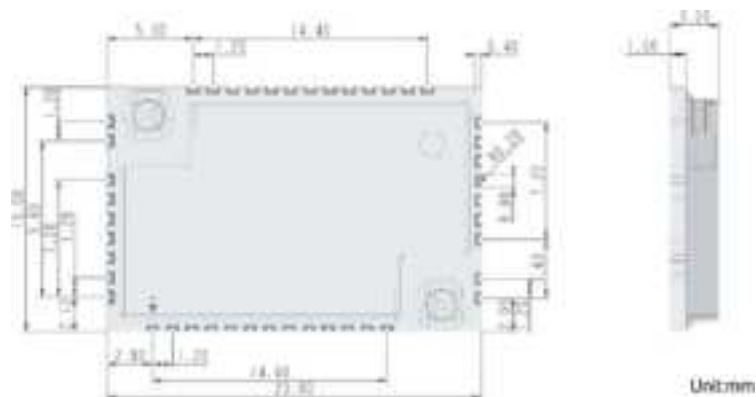
Figure 2: Top and Side Dimensions
