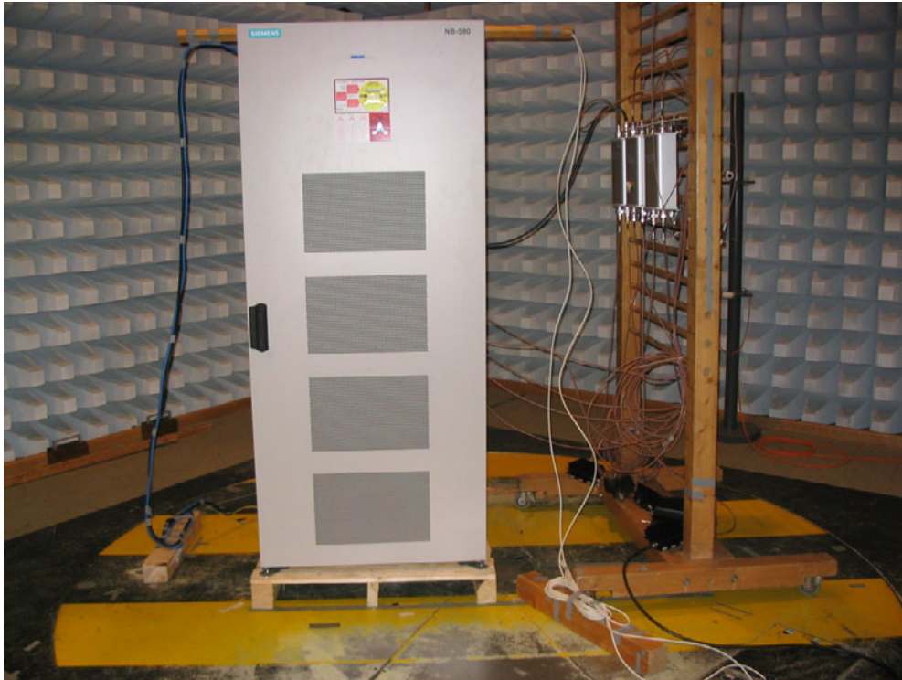
Fig. 28 – Photograph of the anechoic chamber with the EUT
