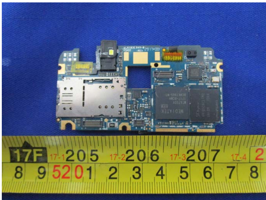
EUT – Main Board Unshield Top View
