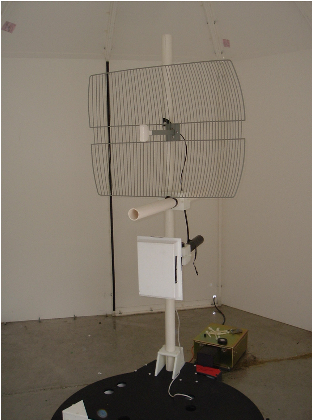
Radiated Emissions Test Setup – 24 dBi Grid
