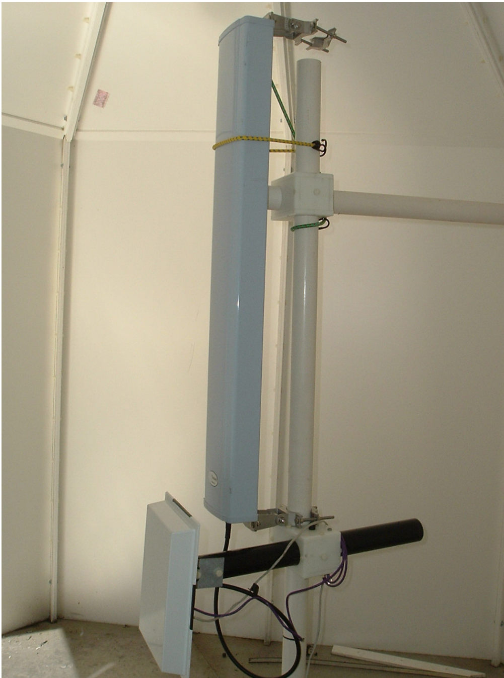
Radiated Emissions Test Setup – 17 dBi Sector
