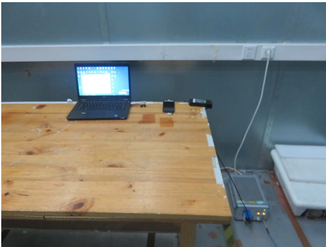
Picture 2 Conducted Emission Test Setup
