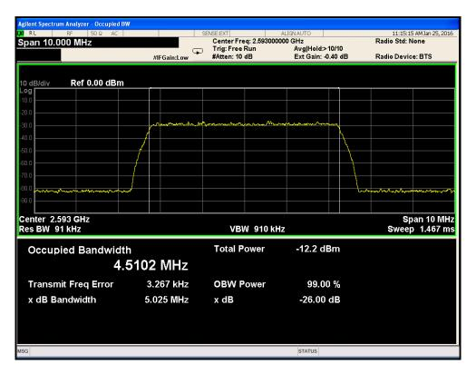
· Input signal bandwidth / 5MHz / 16QAM
