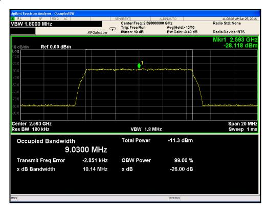
• Input signal bandwidth / 10MHz / 64QAM
