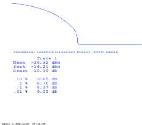
Figure 3-39a: Band 2, Mid Channel PAR, 10 MHz BW, RB = 25 QPSK
