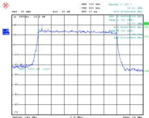
Figure 4-21a: Occupied Bandwidth, Band 5 High Channel, 10MHz BW, RB=50
