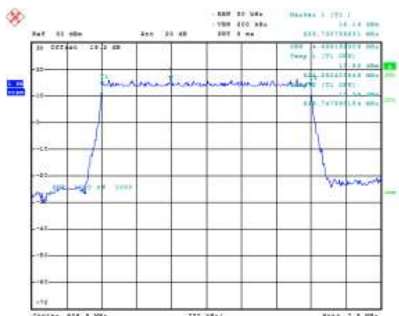
Figure 4-22a: Occupied Bandwidth, Band 5 Low Channel, 5MHz BW, RB=25
