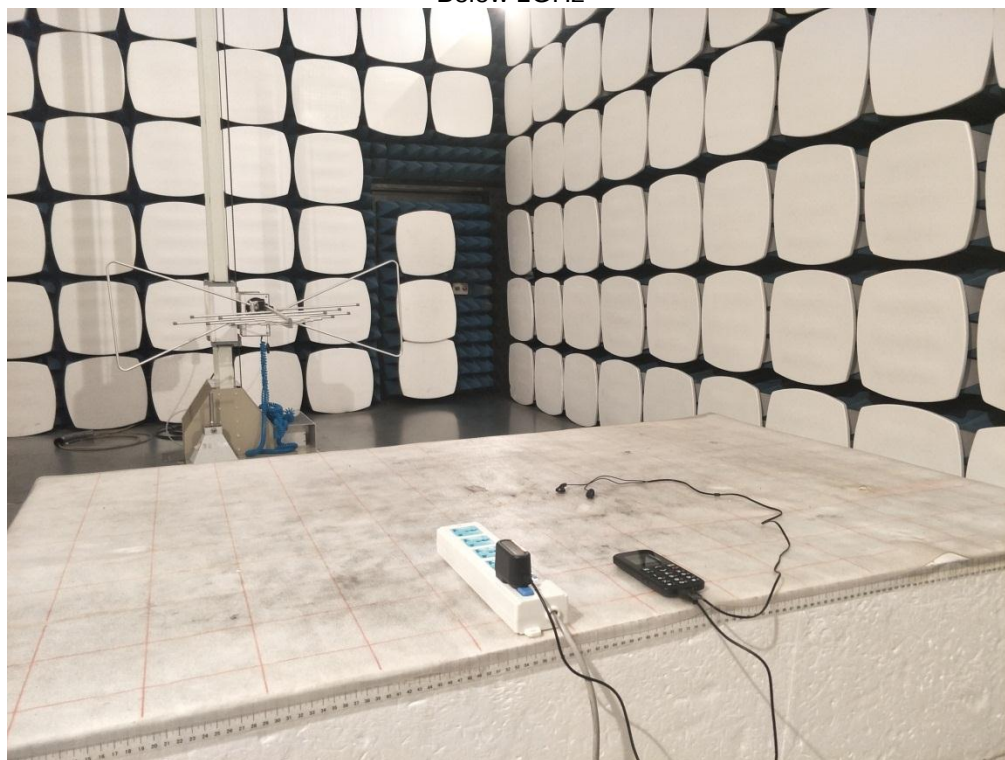
Radiated Emission(for Charging+Recording mode) Below 1GHz
