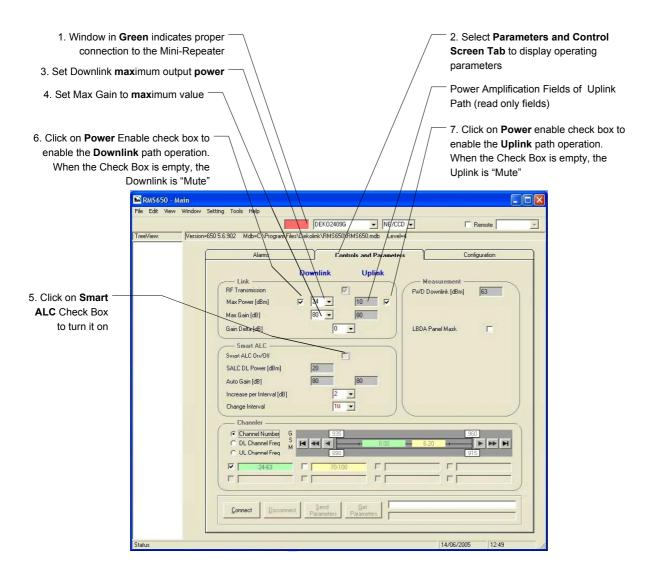
Figure 1: RMS Software - Controls and Parameters Screen
