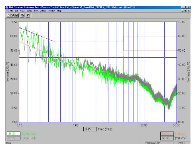
The Handheld in battery charging mode was connected to the Rapid Battery Travel Charger, model number PSM08R-050RIM, part number ASY-07041-001. The ac input to the Rapid Battery Travel Charger was 120 volts, 60 Hz.
