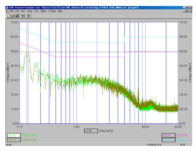
The Handheld in battery charging mode was connected via the detachable USB cable model number HDW-06610-001 to the External Battery Charger. The ac input to the External Battery Charger was 120 volts, 60 Hz.
