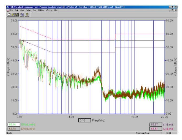
The Handheld in battery charging mode was connected to the Travel Charger, model number PSM05R-050Q, part number ASY-04078-001 via the USB data cable, model number HDW-06610-001. The ac input to the Travel Charger was 120 volts, 60 Hz.
