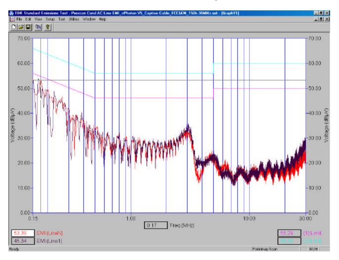
The Handheld in battery charging mode was connected to the Travel Charger, part number ASY-03746-003. The ac input to the Travel Charger was 120 volts, 60 Hz.
