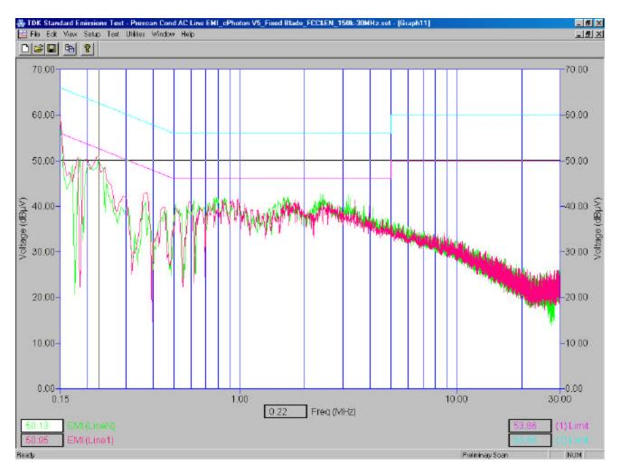
The Handheld in battery charging mode was connected to the North American Travel Charger model number PSM04A-050RIM, ASY-07040-001. The ac input to the North American Travel Charger was 120 volts, 60 Hz.
