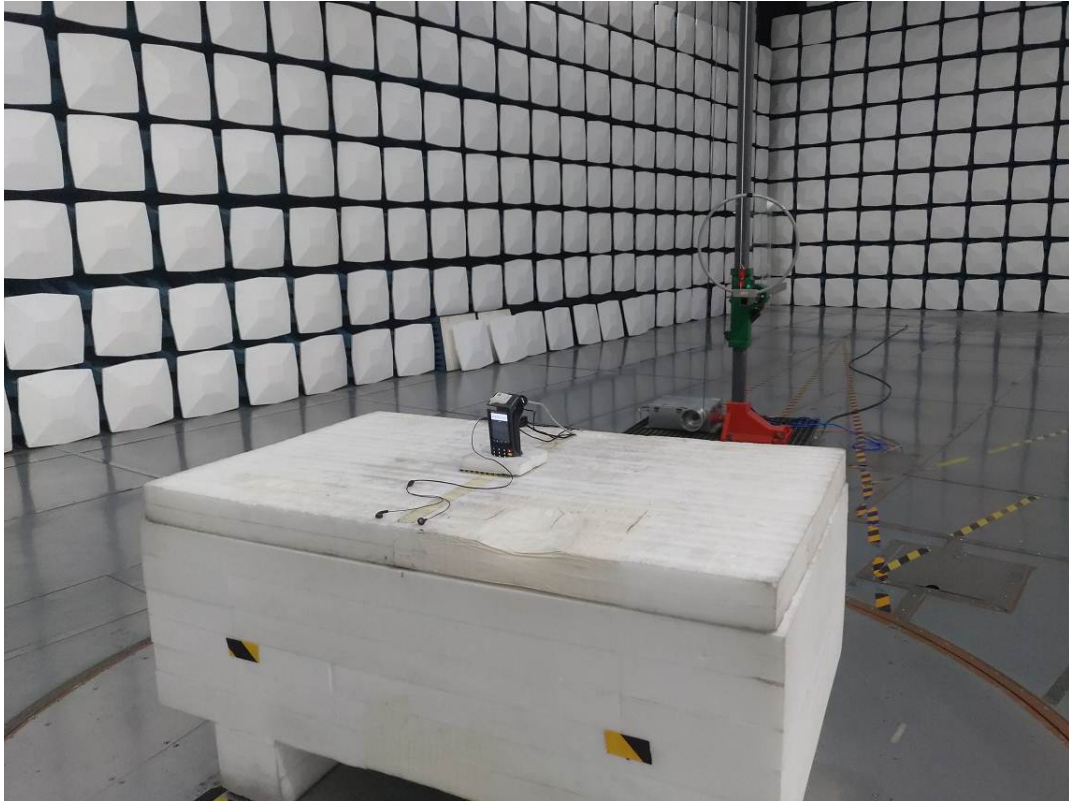
Radiated Emission 9k-30MHz Perpendicular View
