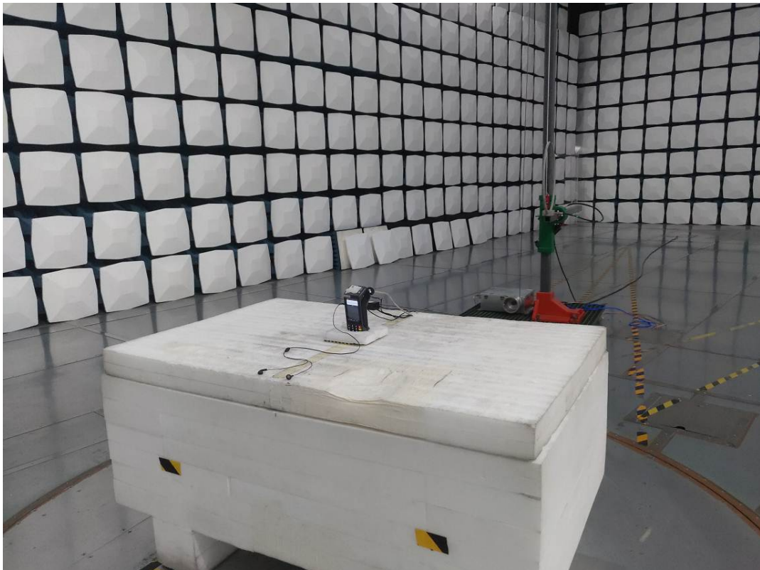
Radiated Emission 9k-30MHz Perpendicular View
