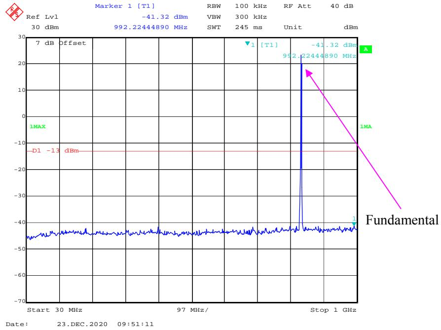
**1 GHz – 10 GHz (QPSK, 1.4 MHz, Middle Channel)**
