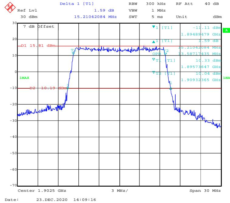
**16-QAM (20 MHz) - 99% Occupied & 26 dB Emissions Bandwidth, High channel**
