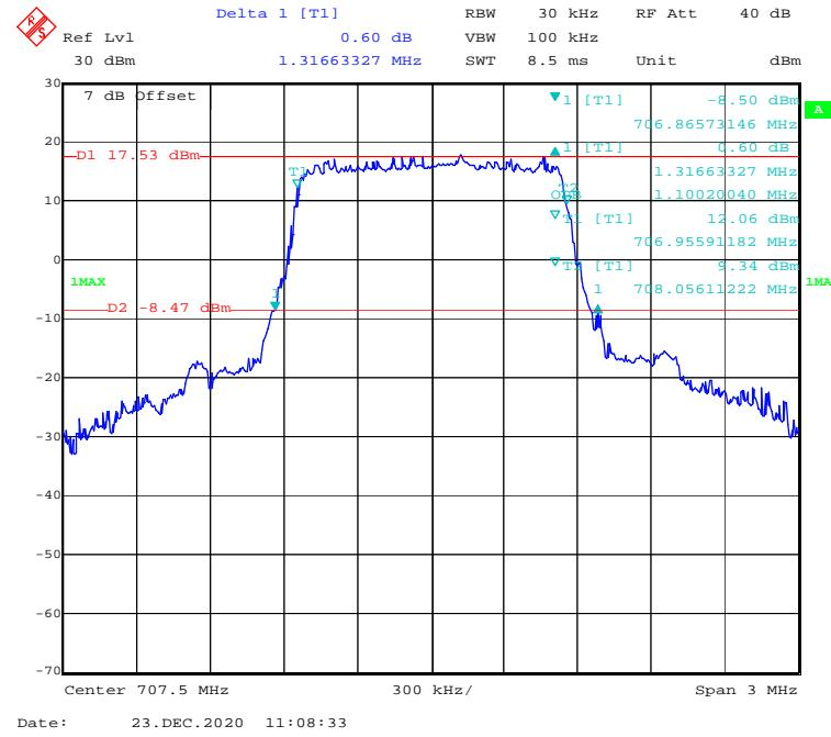
**QPSK (3 MHz) - 99% Occupied & 26 dB Emissions Bandwidth, Middle channel**
