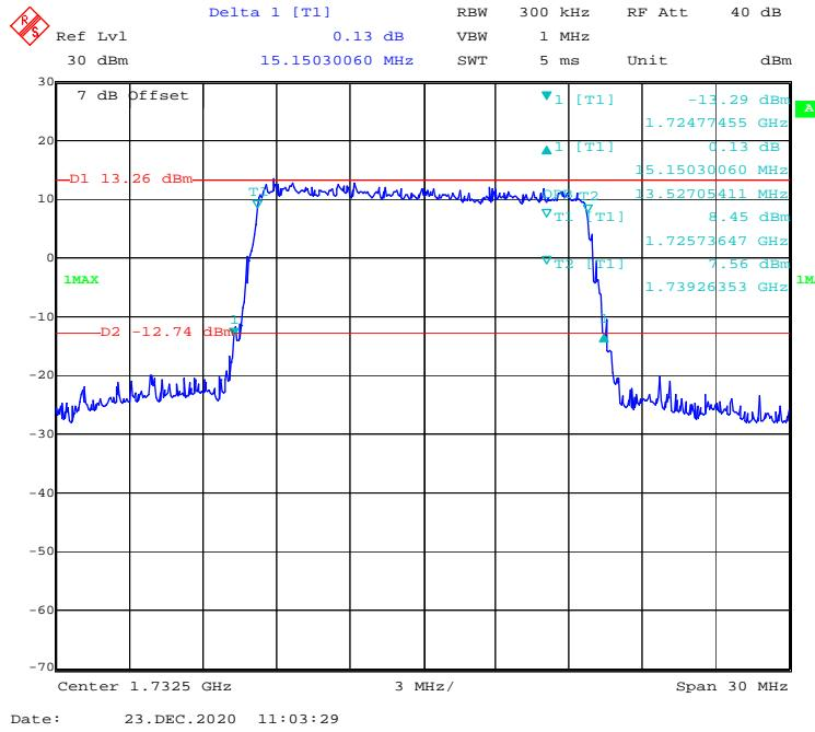
**QPSK (20 MHz) - 99% Occupied & 26 dB Emissions Bandwidth, Middle channel**
