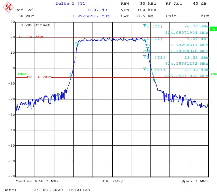
**16-QAM (3.0 MHz) - 99% Occupied & 26 dB Emissions Bandwidth, Low channel**
