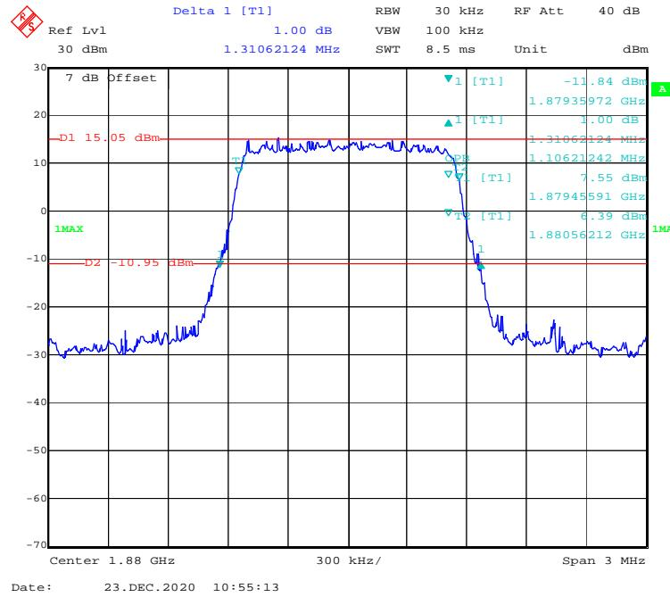
**QPSK (3 MHz) - 99% Occupied & 26 dB Emissions Bandwidth, Middle channel**
