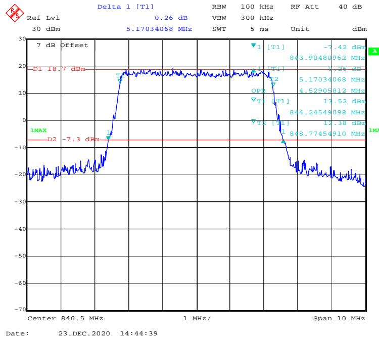
**QPSK (10.0 MHz) - 99% Occupied & 26 dB Emissions Bandwidth, High channel**
