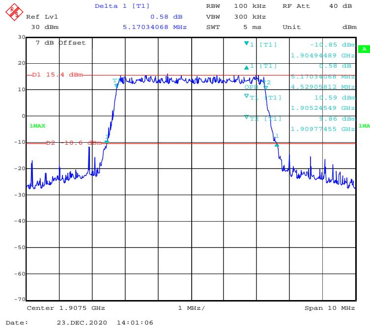
**QPSK (10MHz) - 99% Occupied & 26 dB Emissions Bandwidth, High channel**
