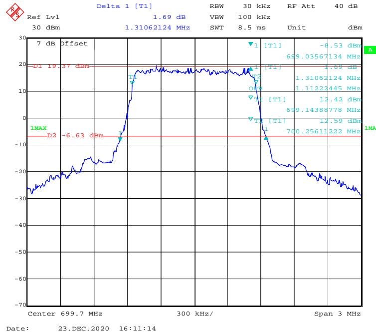
**QPSK (3 MHz) - 99% Occupied & 26 dB Emissions Bandwidth, Low channel**
