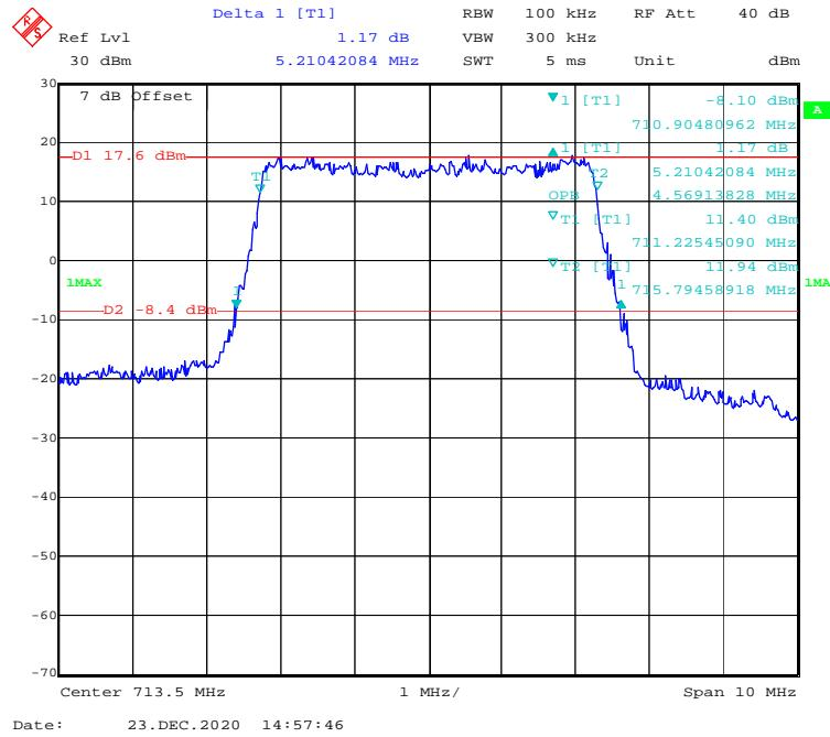
**QPSK (10MHz) - 99% Occupied & 26 dB Emissions Bandwidth, High channel**
