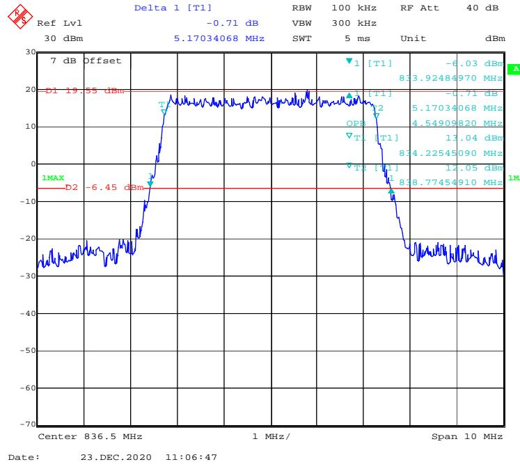
**QPSK (10.0 MHz) - 99% Occupied & 26 dB Emissions Bandwidth, Middle channel**
