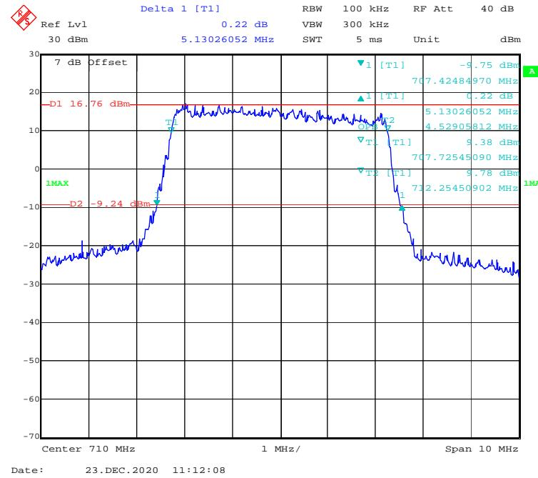
**16-QAM (10 MHz) - 99% Occupied & 26 dB Emissions Bandwidth, Middle channel**
