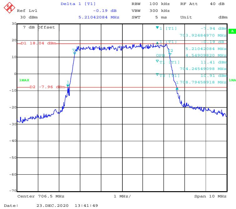
**QPSK (10MHz) - 99% Occupied & 26 dB Emissions Bandwidth, Low channel**
