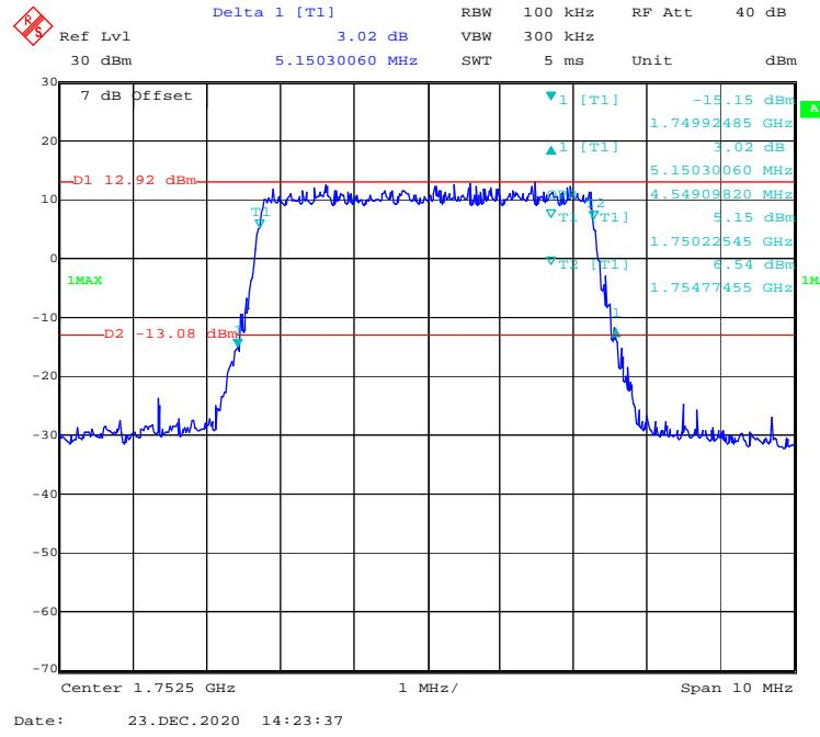
**QPSK (10 MHz) - 99% Occupied & 26 dB Emissions Bandwidth, High channel**
