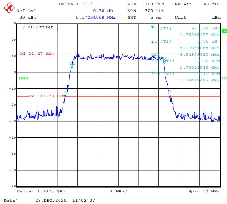
**16-QAM (10 MHz) - 99% Occupied & 26 dB Emissions Bandwidth, Middle channel**
