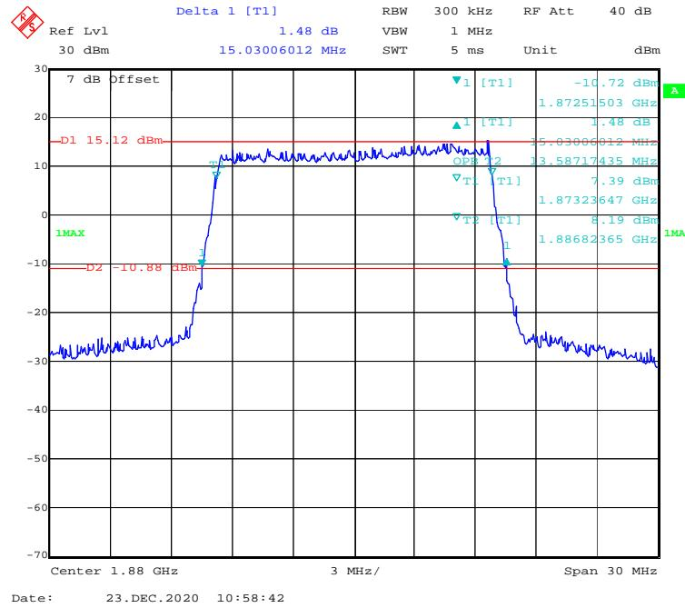
**16-QAM (20 MHz) - 99% Occupied & 26 dB Emissions Bandwidth, Middle channel**
