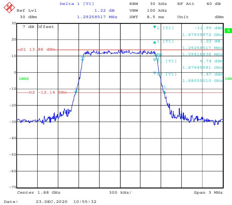
**16-QAM (3 MHz) - 99% Occupied & 26 dB Emissions Bandwidth, Middle channel**
