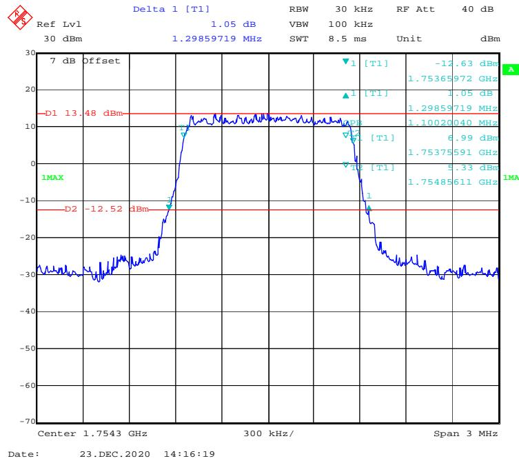
**QPSK (3 MHz) - 99% Occupied & 26 dB Emissions Bandwidth, High channel**
