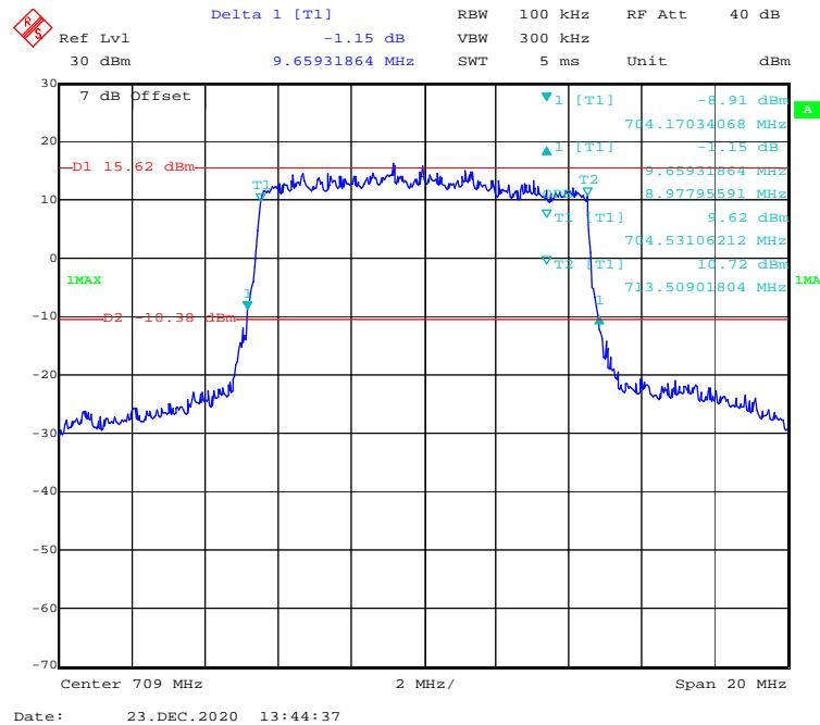
**QPSK (5 MHz) - 99% Occupied & 26 dB Emissions Bandwidth, Middle channel**
