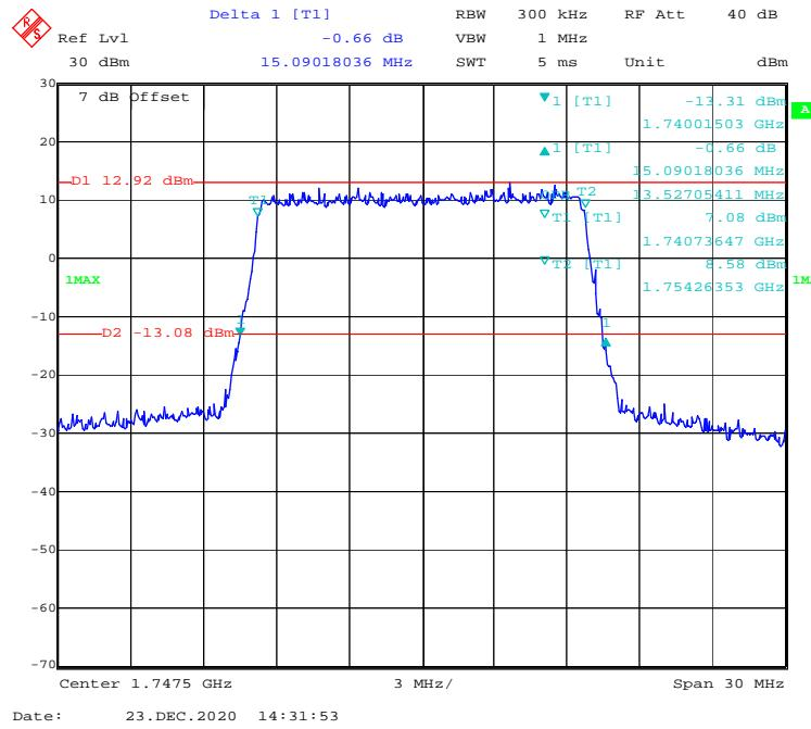
**16-QAM (20 MHz) - 99% Occupied & 26 dB Emissions Bandwidth, High channel**
