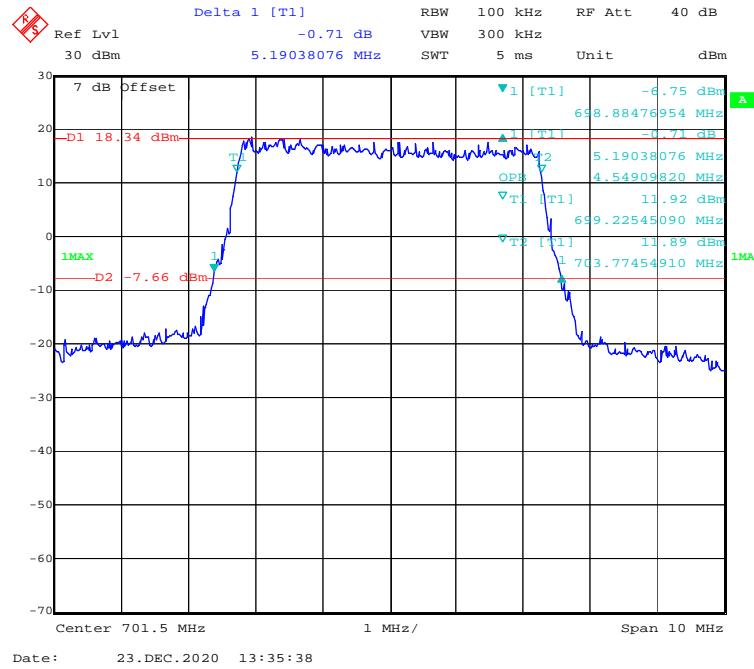
**QPSK (10MHz) - 99% Occupied & 26 dB Emissions Bandwidth, Low channel**
