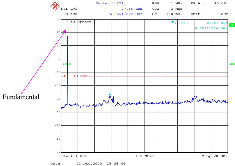
**30 MHz - 1 GHz (10 MHz, QPSK, High Channel)**
