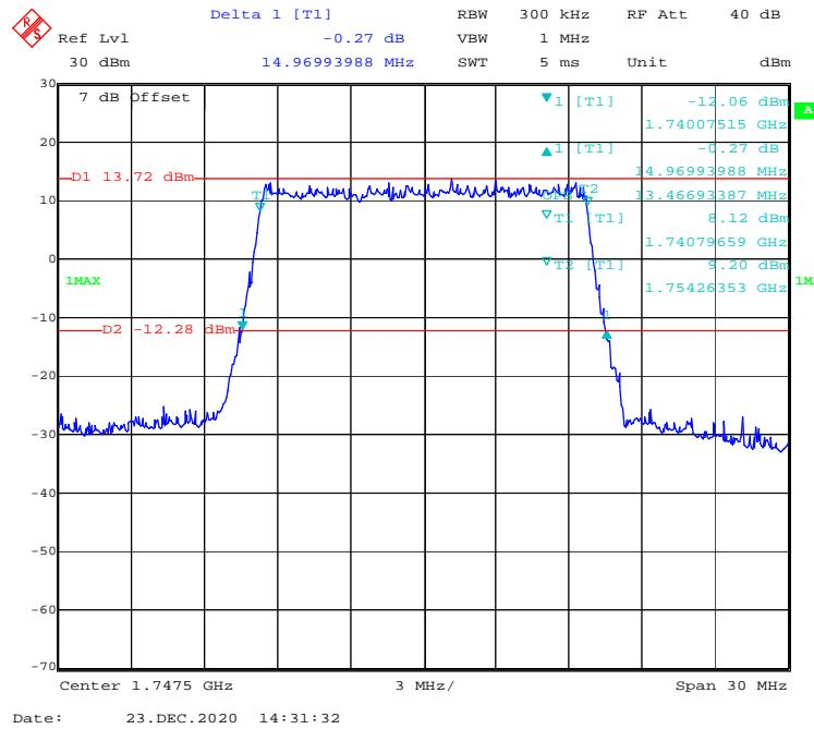
**QPSK (20 MHz) - 99% Occupied & 26 dB Emissions Bandwidth, High channel**
