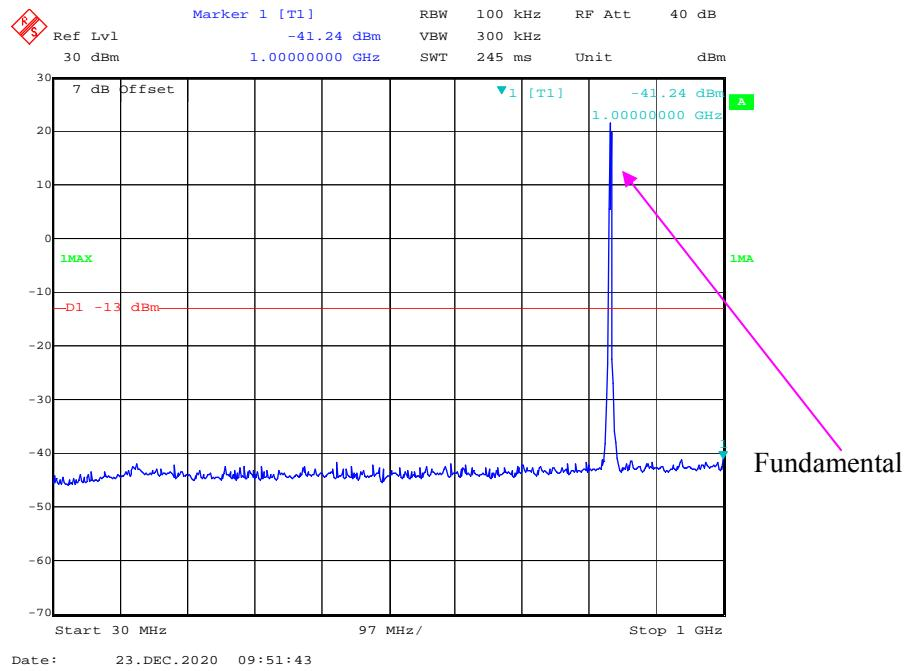
**1 GHz – 10 GHz (QPSK, 3.0 MHz, Middle Channel)**
