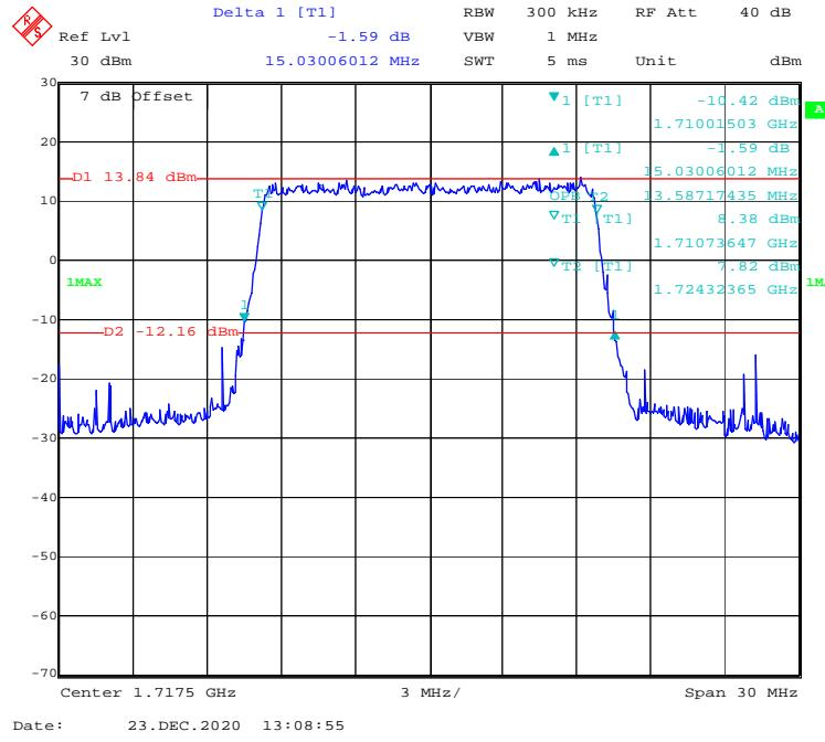
**QPSK (20 MHz) - 99% Occupied & 26 dB Emissions Bandwidth, Low channel**
