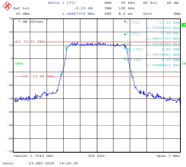
**16-QAM (3 MHz) - 99% Occupied & 26 dB Emissions Bandwidth, High channel**
