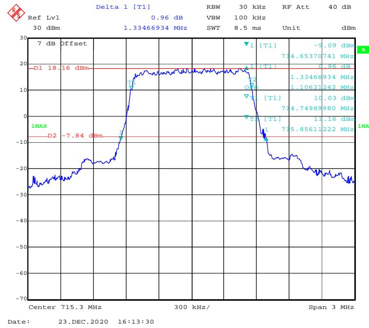
**QPSK (3 MHz) - 99% Occupied & 26 dB Emissions Bandwidth, High channel**
