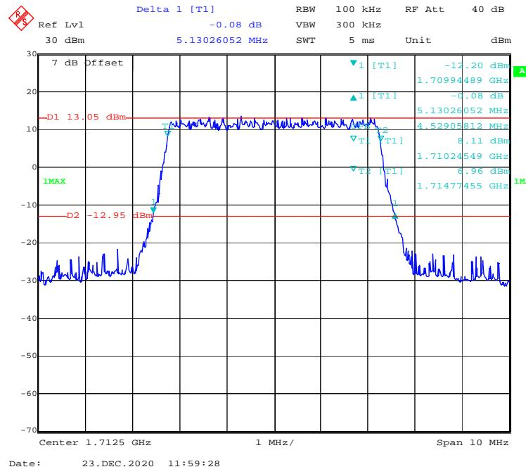
**QPSK (10 MHz) - 99% Occupied & 26 dB Emissions Bandwidth, Low channel**
