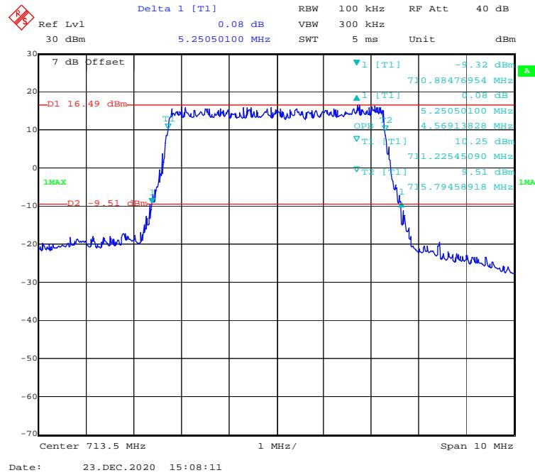
**16-QAM (10 MHz) - 99% Occupied & 26 dB Emissions Bandwidth, High channel**
