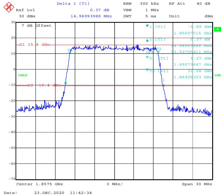
**16-QAM (20 MHz) - 99% Occupied & 26 dB Emissions Bandwidth, Low channel**
