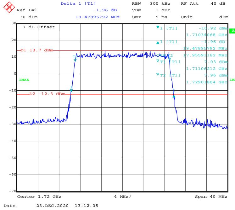
**QPSK (1.4 MHz) - 99% Occupied & 26 dB Emissions Bandwidth, Middle channel**
