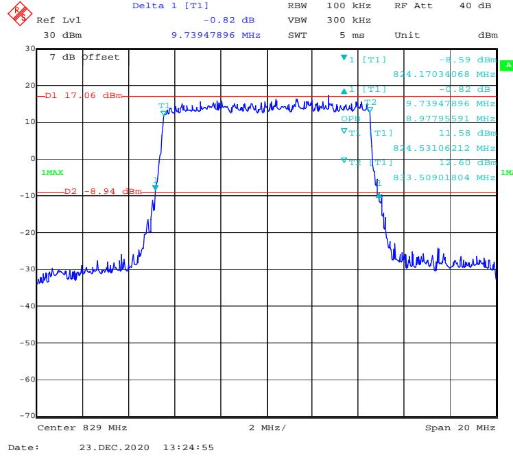
**QPSK (1.4 MHz) - 99% Occupied & 26 dB Emissions Bandwidth, Middle channel**
