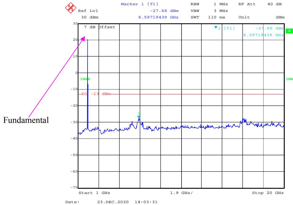
**30 MHz - 1 GHz (10 MHz, QPSK, High Channel)**
