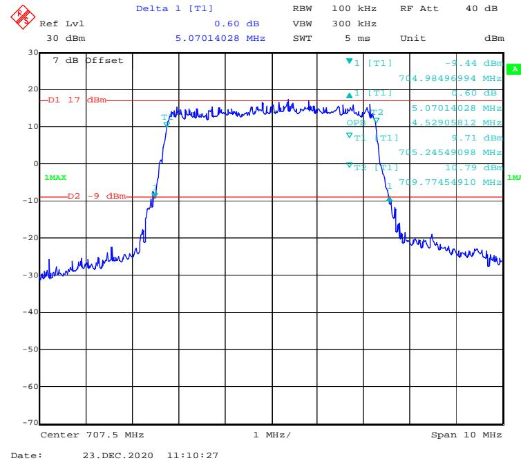
**16-QAM (10 MHz) - 99% Occupied & 26 dB Emissions Bandwidth, Middle channel**
