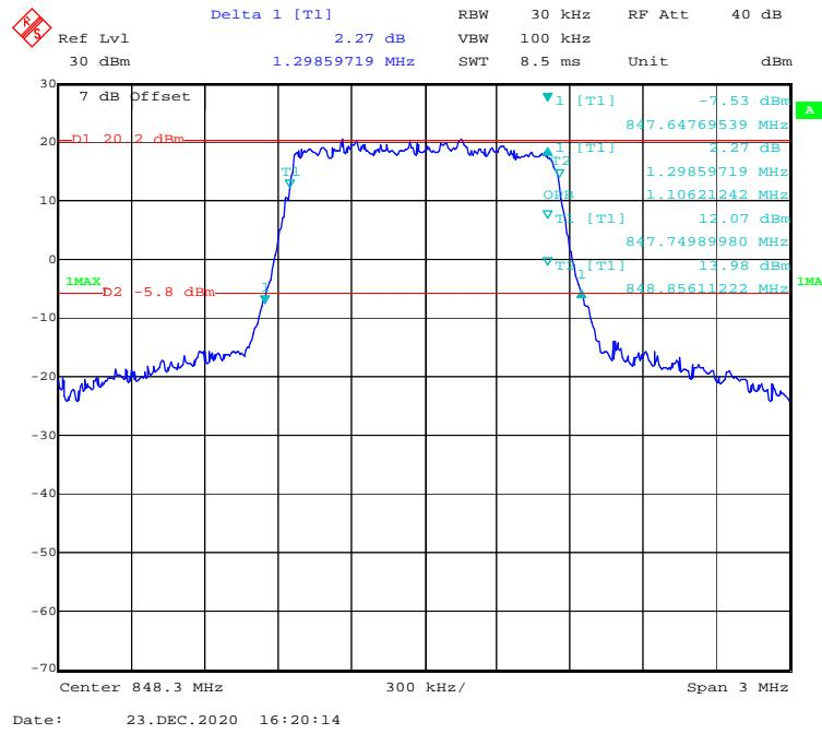
**QPSK (3.0 MHz) - 99% Occupied & 26 dB Emissions Bandwidth, High channel**
