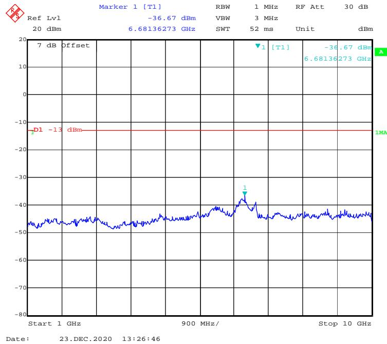
**30 MHz - 1 GHz (16QAM, 1.4 MHz, Low Channel)**
