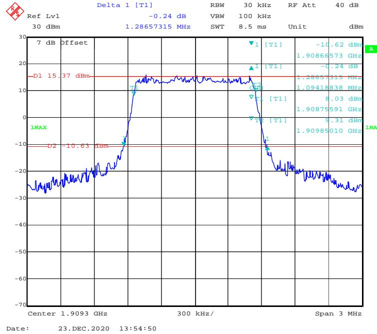
**16-QAM (3 MHz) - 99% Occupied & 26 dB Emissions Bandwidth, High channel**
