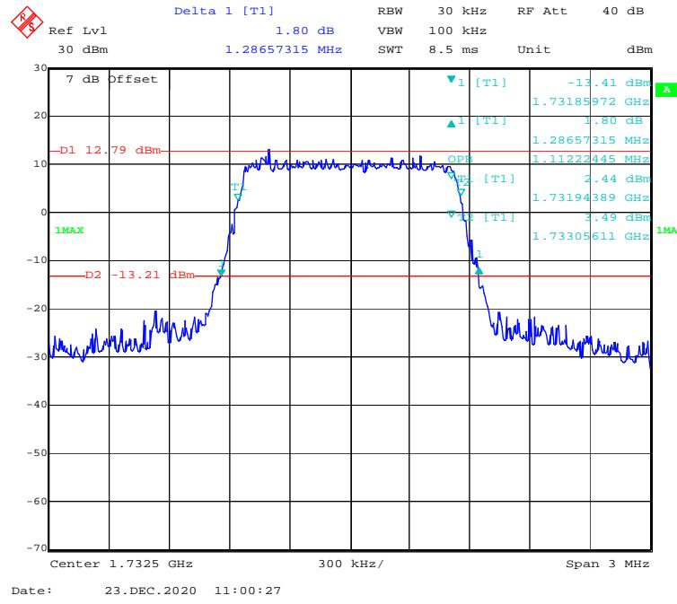
**16-QAM (3 MHz) - 99% Occupied & 26 dB Emissions Bandwidth, Middle channel**
