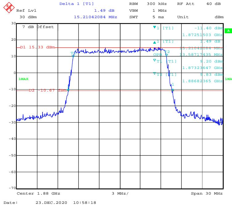
**QPSK (20 MHz) - 99% Occupied & 26 dB Emissions Bandwidth, Middle channel**
