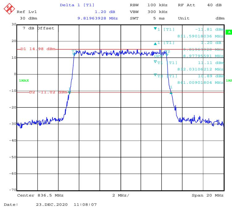
**16-QAM (1.4 MHz) - 99% Occupied & 26 dB Emissions Bandwidth, High channel**
