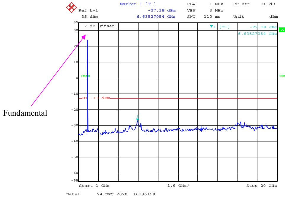
**30 MHz – 1GHz WCDMA (HSPA+) Mode , Middle channel**
