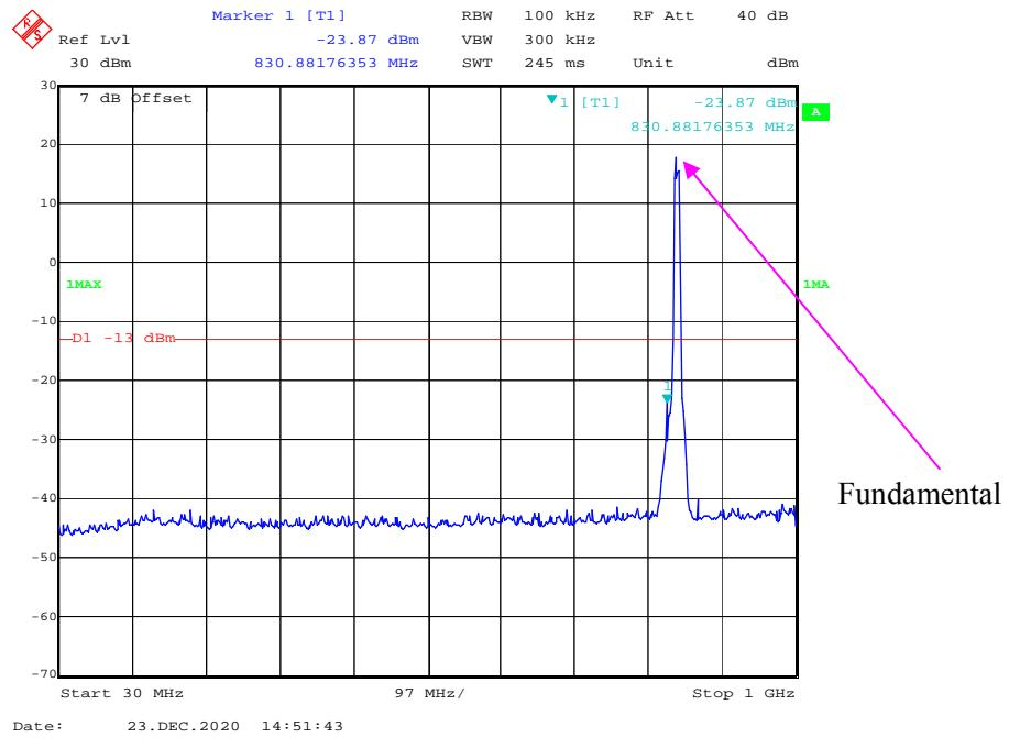
**1 GHz – 10 GHz (16QAM, 10.0 MHz, High Channel)**
