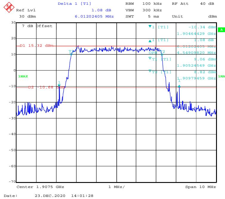
**16-QAM (10 MHz) - 99% Occupied & 26 dB Emissions Bandwidth, High channel**
