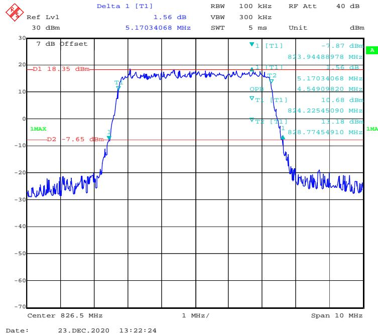
**16-QAM (10.0 MHz) - 99% Occupied & 26 dB Emissions Bandwidth, Low channel**
