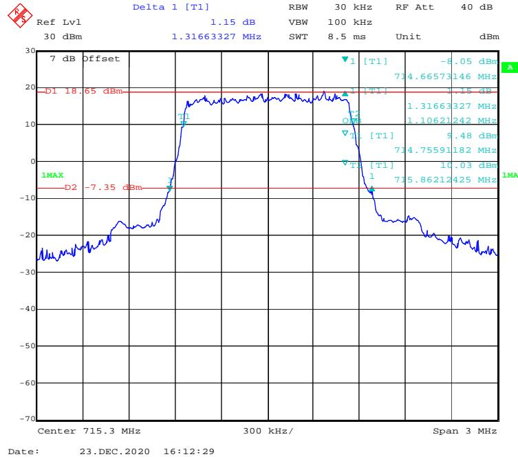
**16-QAM (3 MHz) - 99% Occupied & 26 dB Emissions Bandwidth, High channel**
