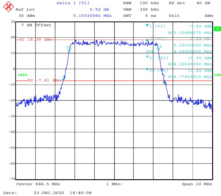
**16-QAM (10.0 MHz) - 99% Occupied & 26 dB Emissions Bandwidth, High channel**
