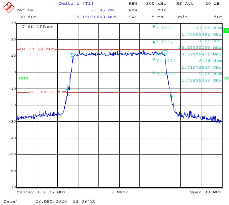
**16-QAM (20 MHz) - 99% Occupied & 26 dB Emissions Bandwidth, Low channel**
