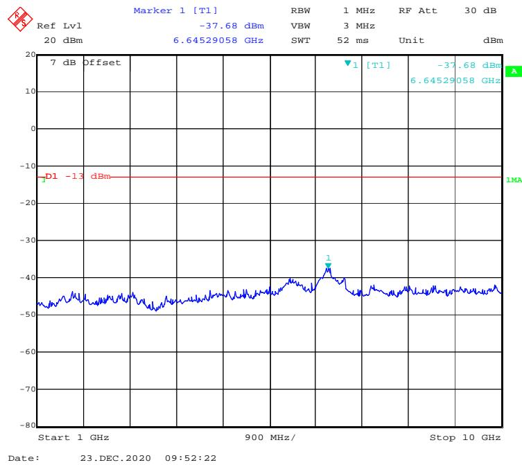
**30 MHz - 1 GHz (QPSK, 10.0 MHz, Middle Channel)**
