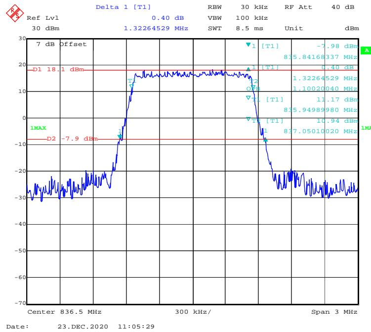
**16-QAM (3.0 MHz) - 99% Occupied & 26 dB Emissions Bandwidth, Middle channel**
