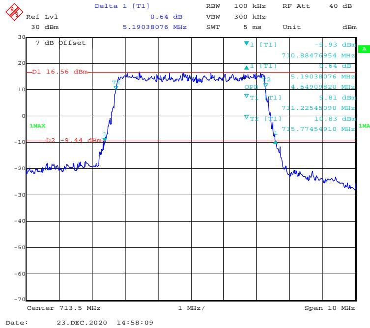
**16-QAM (10 MHz) - 99% Occupied & 26 dB Emissions Bandwidth, High channel**
