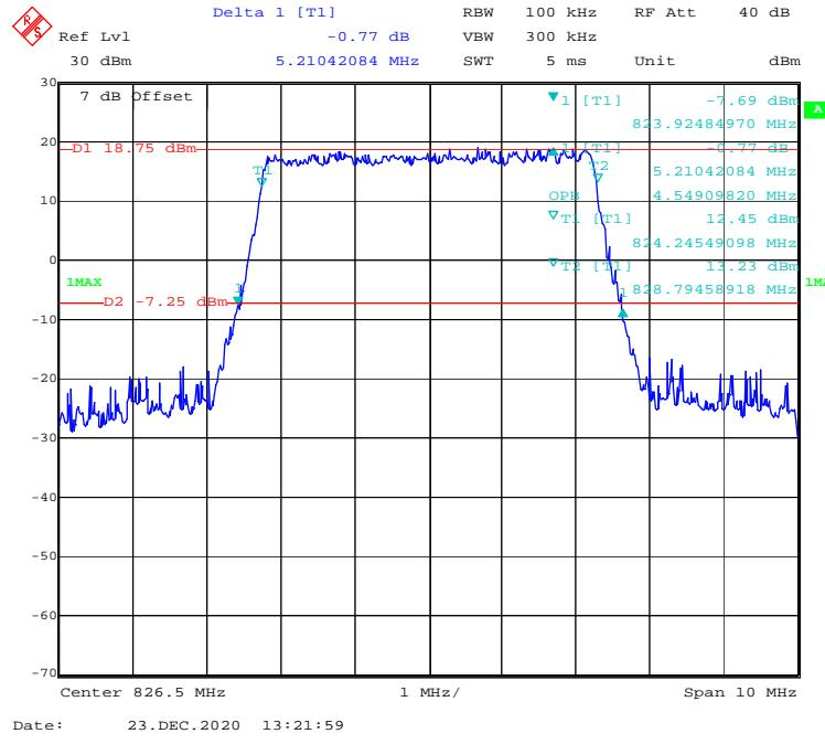
**QPSK (10.0 MHz) - 99% Occupied & 26 dB Emissions Bandwidth, Low channel**
