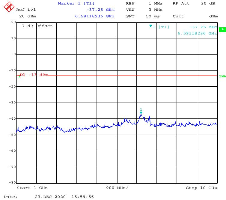
**30 MHz - 1 GHz (1.4 MHz, 16-QAM, Low Channel)**
