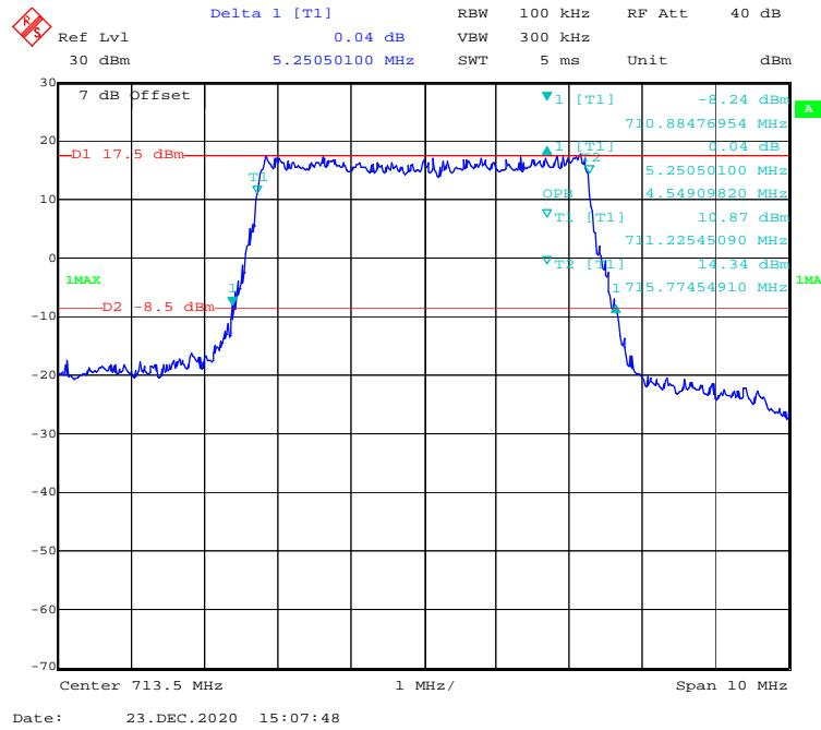
**QPSK (10MHz) - 99% Occupied & 26 dB Emissions Bandwidth, High channel**
