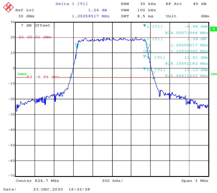
**QPSK (3.0 MHz) - 99% Occupied & 26 dB Emissions Bandwidth, Low channel**
