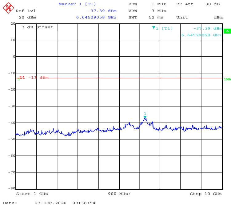
**30 MHz - 1 GHz (QPSK, 1.4 MHz, High Channel)**
