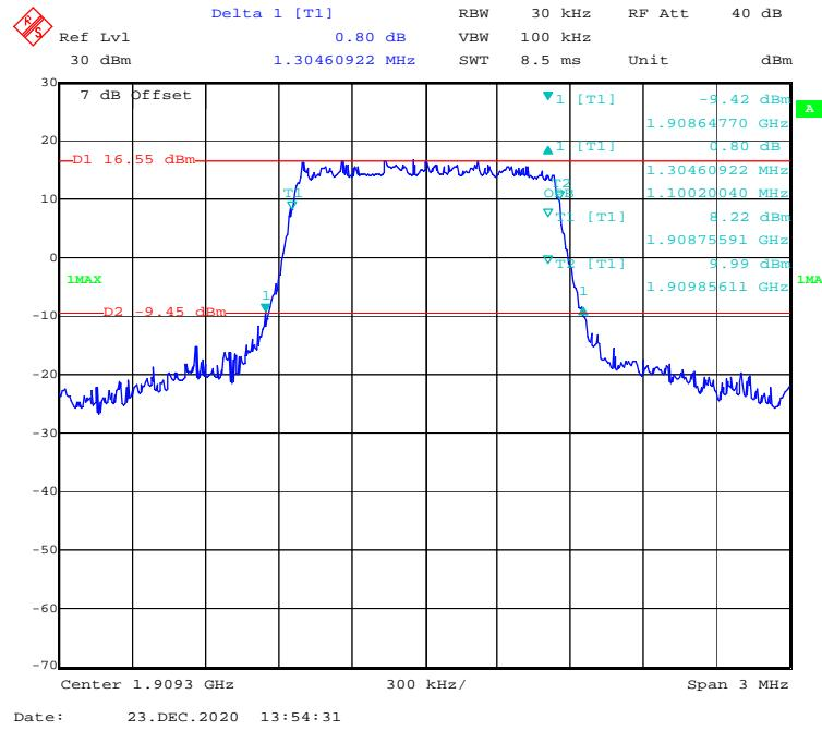
**QPSK (3 MHz) - 99% Occupied & 26 dB Emissions Bandwidth, High channel**
