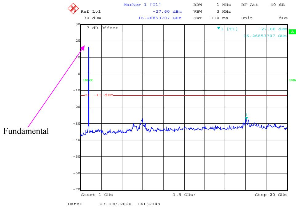
**30 MHz - 1 GHz (20 MHz, QPSK, High Channel)**
