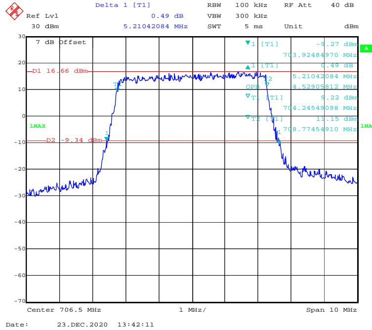
**16-QAM (10 MHz) - 99% Occupied & 26 dB Emissions Bandwidth, Low channel**
