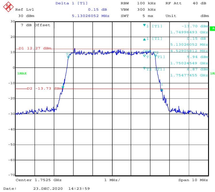
**16-QAM (10 MHz) - 99% Occupied & 26 dB Emissions Bandwidth, High channel**
