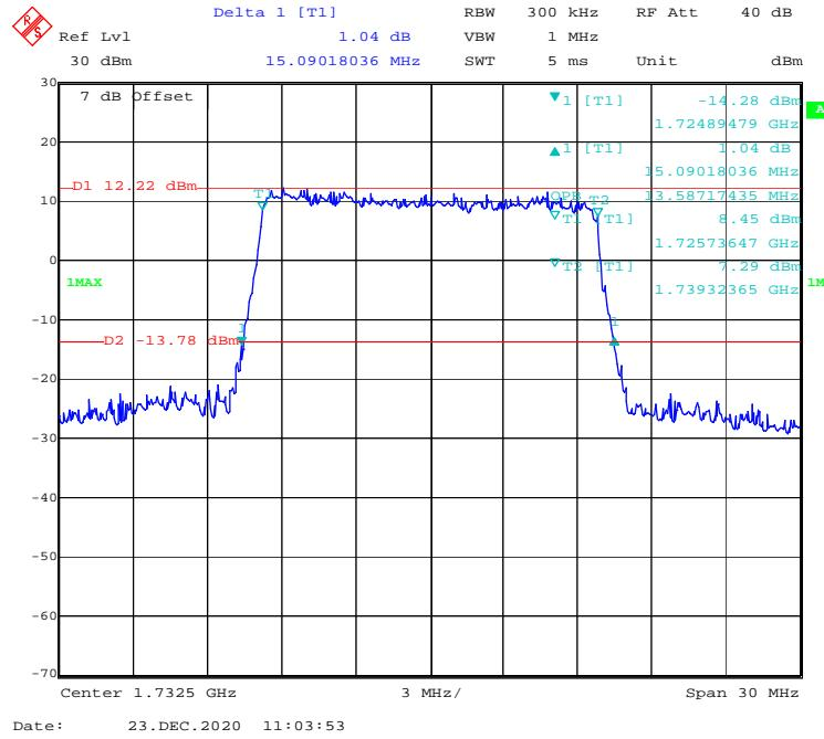
**16-QAM (20 MHz) - 99% Occupied & 26 dB Emissions Bandwidth, Middle channel**
