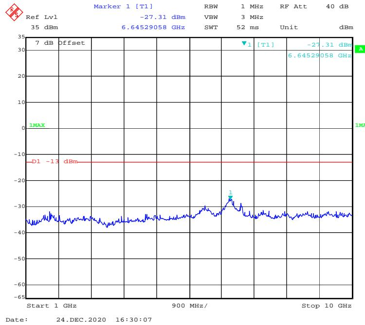
**30 MHz – 1GHz WCDMA (Rel 99) Mode, High channel**
