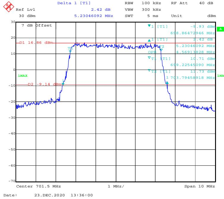
**16-QAM (10 MHz) - 99% Occupied & 26 dB Emissions Bandwidth, Low channel**
