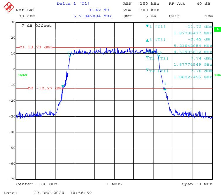
**16-QAM (10 MHz) - 99% Occupied & 26 dB Emissions Bandwidth, Middle channel**
