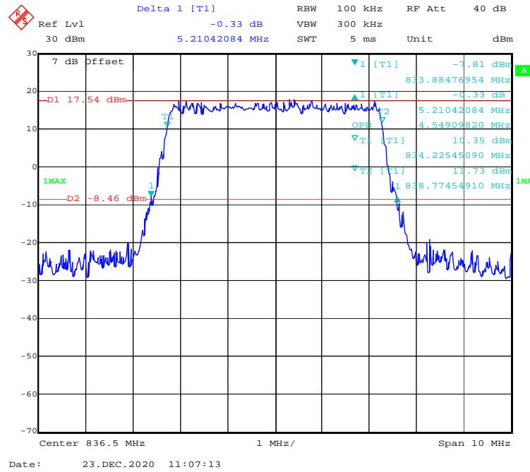
**16-QAM (10.0 MHz) - 99% Occupied & 26 dB Emissions Bandwidth, Middle channel**
