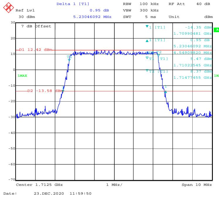
**16-QAM (10 MHz) - 99% Occupied & 26 dB Emissions Bandwidth, Low channel**
