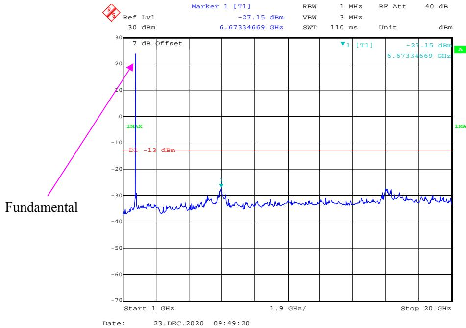
**30 MHz - 1 GHz (5 MHz, 16-QAM, Middle Channel)**
