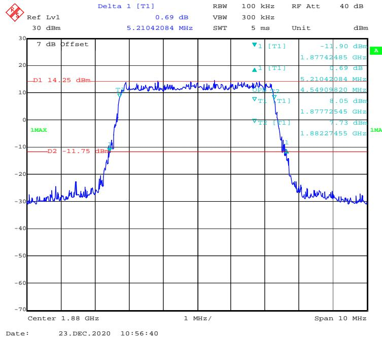
**QPSK (10MHz) - 99% Occupied & 26 dB Emissions Bandwidth, Middle channel**
