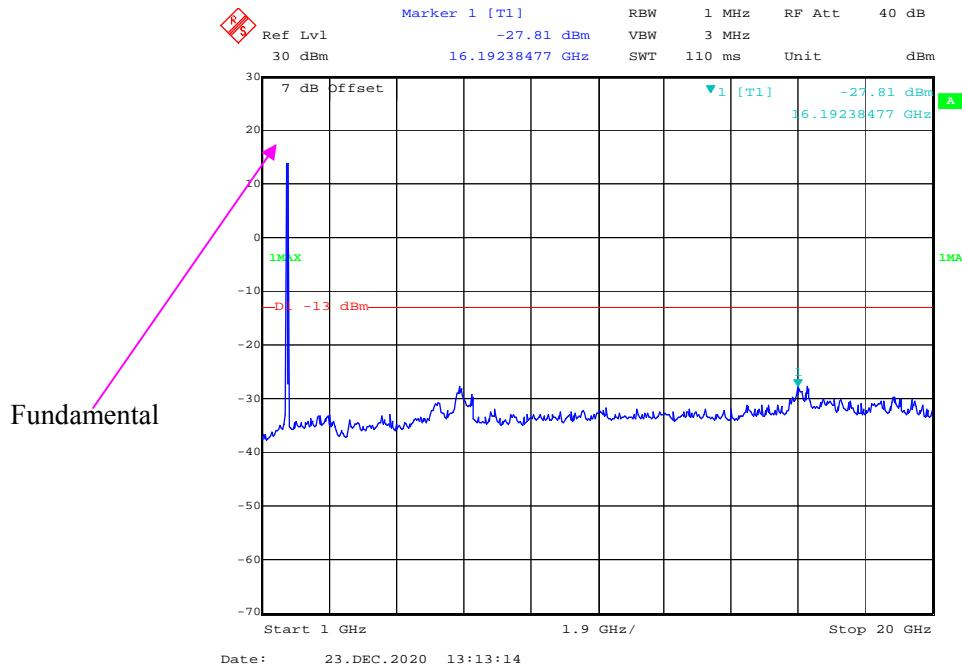
**30 MHz - 1 GHz (1.4 MHz, QPSK, Middle Channel)**
