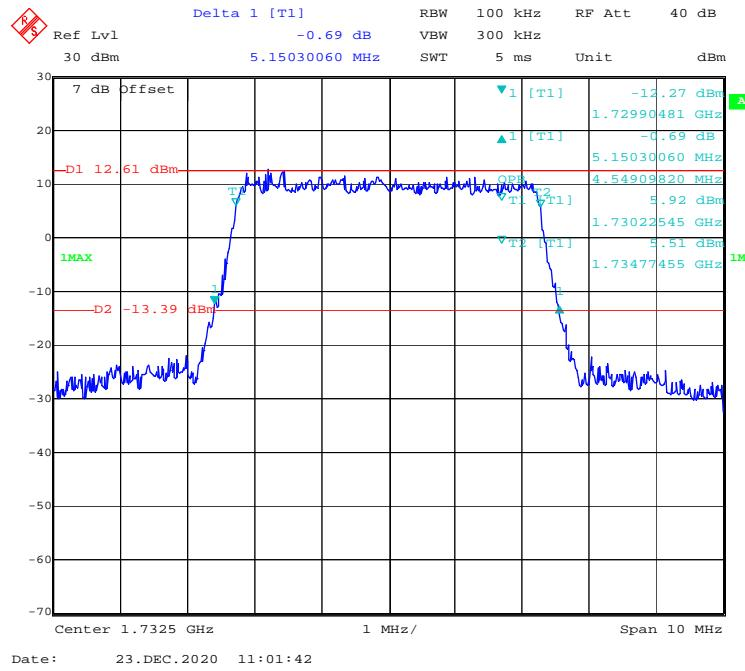
**QPSK (10 MHz) - 99% Occupied & 26 dB Emissions Bandwidth, Middle channel**
