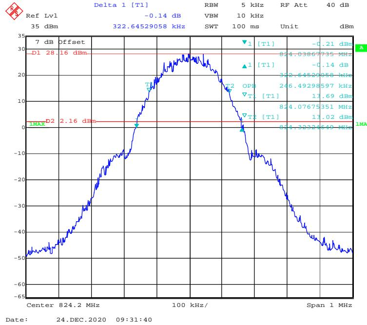
**99% Occupied & 26 dB Emissions Bandwidth for GPRS (GMSK) Middle channel**
