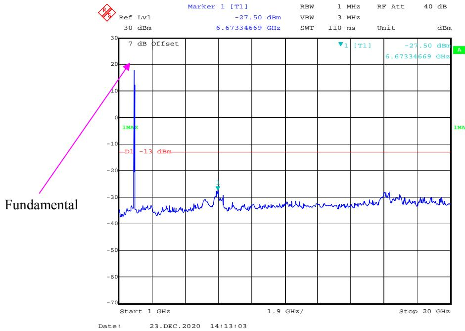
**LTE Band 4:****30 MHz - 1 GHz (1.4 MHz, QPSK, Low Channel)**
