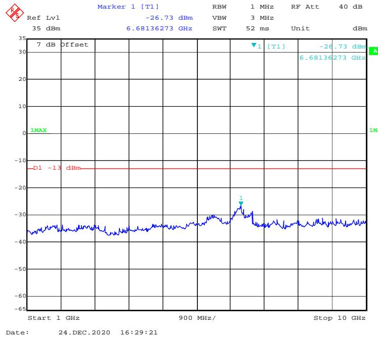
**30 MHz – 1GHz WCDMA (HSUPA) Mode, Middle channel**
