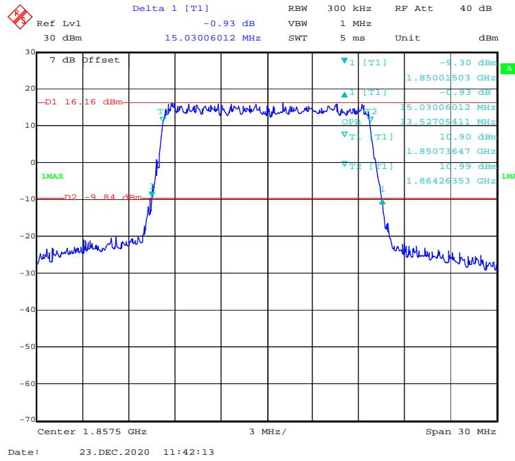
**QPSK (20 MHz) - 99% Occupied & 26 dB Emissions Bandwidth, Low channel**
