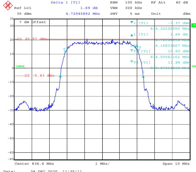
**99% Occupied & 26 dB Emissions Bandwidth for WCDMA (HSUPA) High channel**
