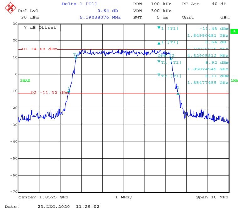
**16-QAM (10 MHz) - 99% Occupied & 26 dB Emissions Bandwidth, Low channel**
