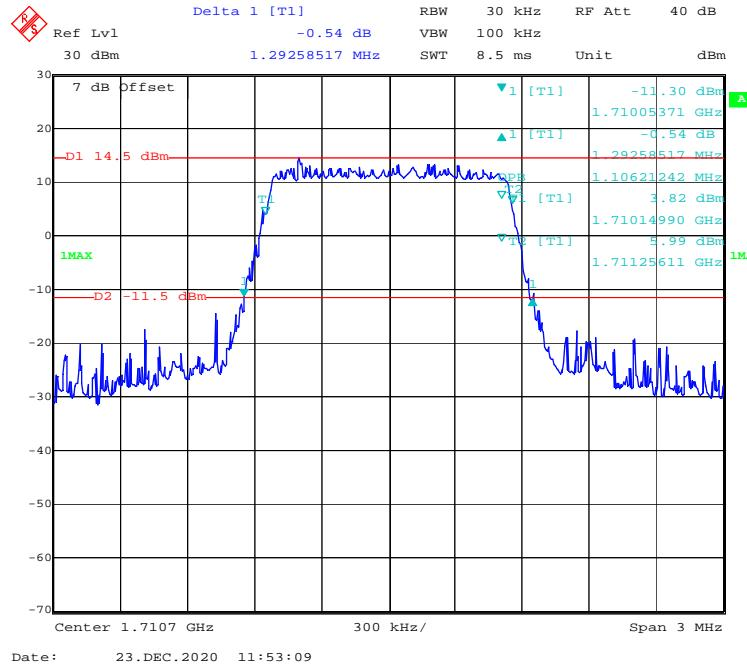
**16-QAM (3 MHz) - 99% Occupied & 26 dB Emissions Bandwidth, Low channel**
