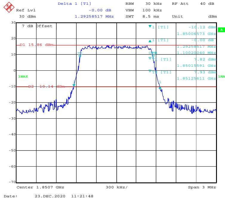
**QPSK (3 MHz) - 99% Occupied & 26 dB Emissions Bandwidth, Low channel**
