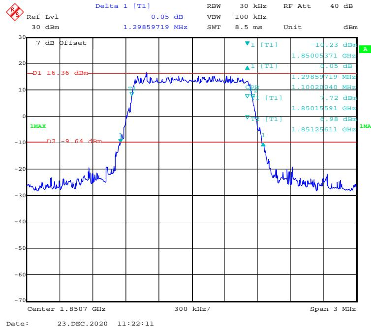
**16-QAM (3 MHz) - 99% Occupied & 26 dB Emissions Bandwidth, Low channel**
