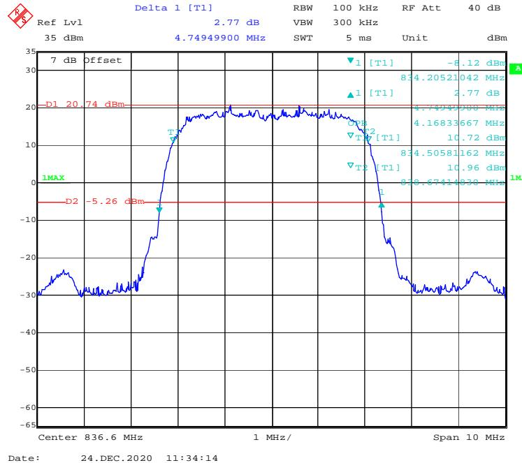
**99% Occupied & 26 dB Emissions Bandwidth for WCDMA (HSDPA) High channel**
