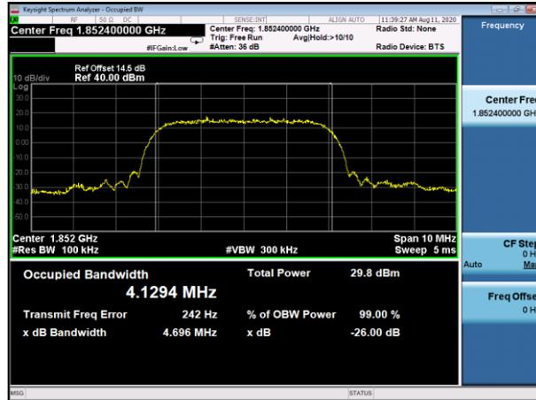
(Plot B1: WCDMA 1900MHz Channel = 9262 Occupied bandwidth)
