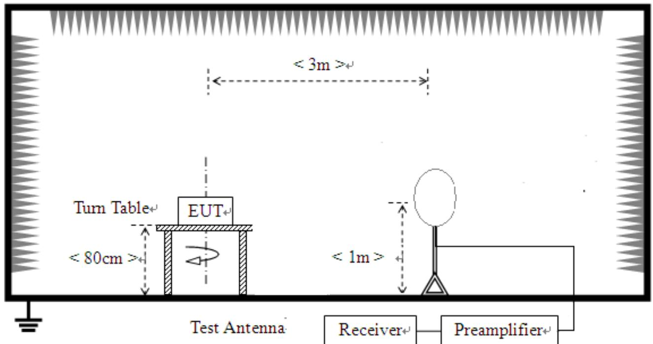
For radiated emissions from 30MHz to 1GHz
