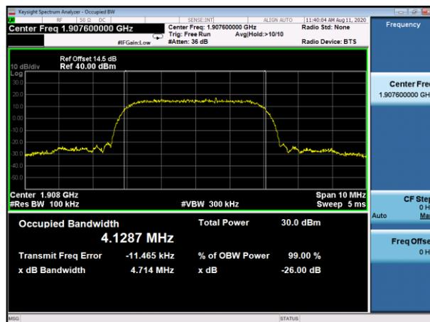
(Plot B3: WCDMA 1900MHz Channel = 9538 Occupied bandwidth)
