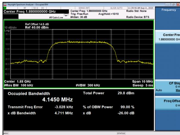
(Plot B2: WCDMA 1900MHz Channel = 9400 Occupied bandwidth)
