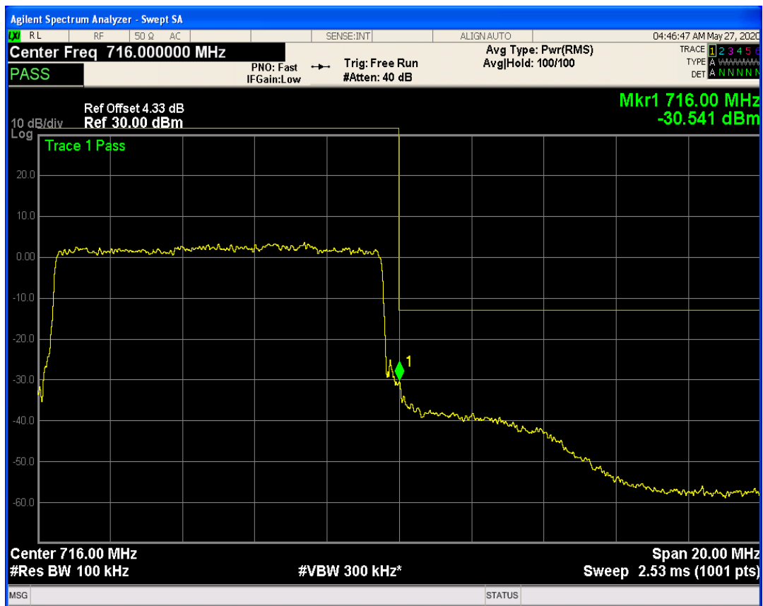
LTE Band17 QAM16 BW=10MHz Channel=23800 RB Size=1 Position=#Max
