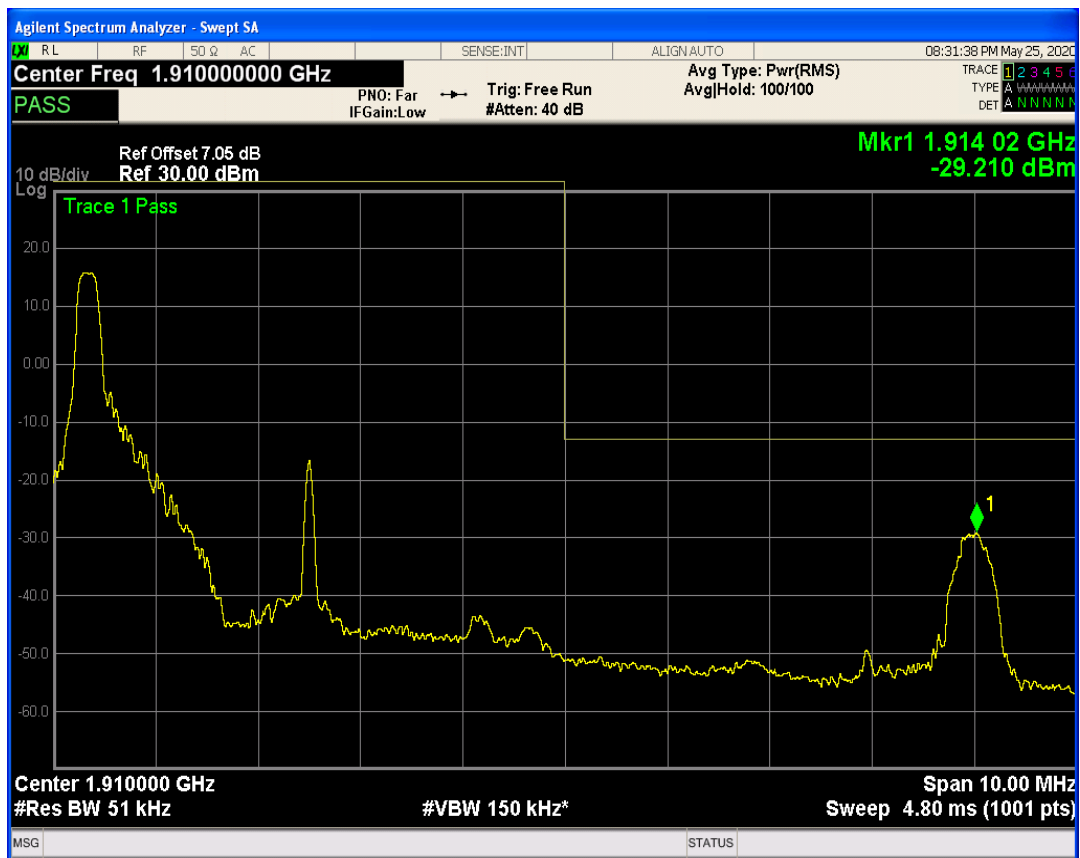
LTE Band2 QAM16 BW=5MHz Channel=19175 RB Size=1 Position=#Max
