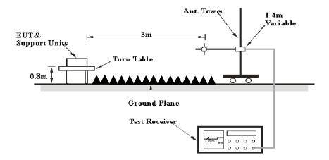
The radiated emission tests were performed at the 3 meters in chamber test site, using the setup accordance with the ANSI C63.4-2014. The specification used was the FCC Part 15.109 Class B limits.
