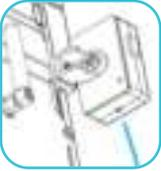
Steps to insert filament: Insert the filament into the hole of the filament runout sensor until it reaches the end. When the consumables cannot be inserted any further, complete the step of inserting filament.
